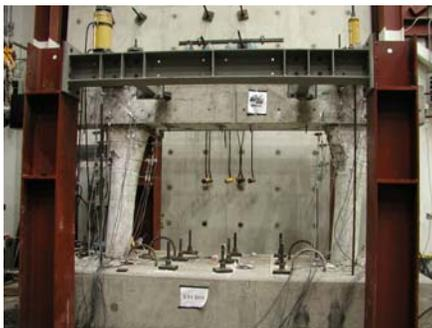
(a) Large drift and displacement before stopping the testing of LFCD1S
