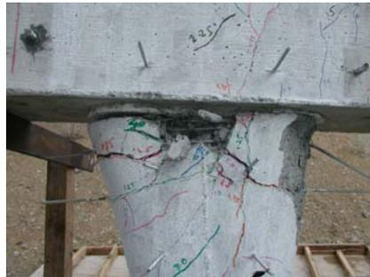
**Figure 9 Damaged flare after the failure of SFCD3**
