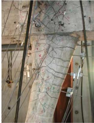
(a) Final condition of LFCD1S after the test
