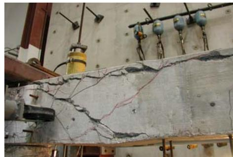
(b) Beam shear failure in SFCD2S
