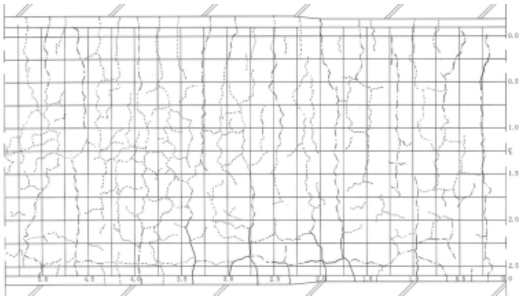
Figure 3 Crack Diagram Produced by Close-Range Direct Visual Inspection
