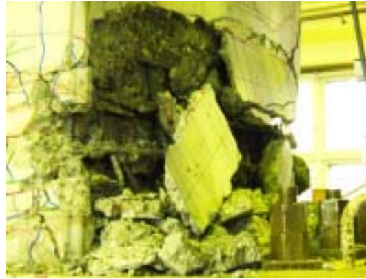
Photo4 Damage condition of the 2.0-R-5 specimen
