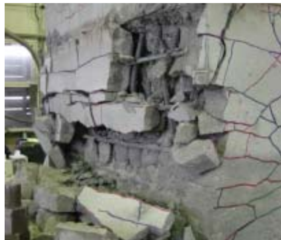
Photo6 Damage condition of the 2.0-M-7 specimen
