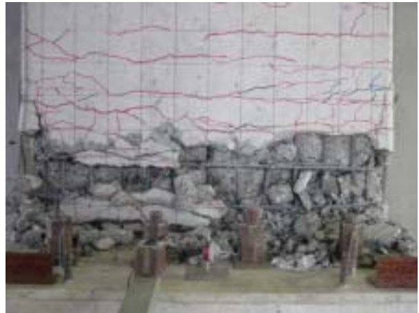
Photo3 Damage condition of the 2.0-R-3 specimen
