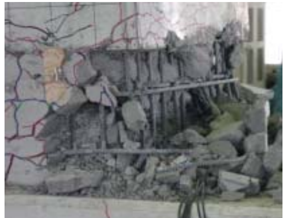
Photo5 Damage condition of the 2.0-M-5 specimen
