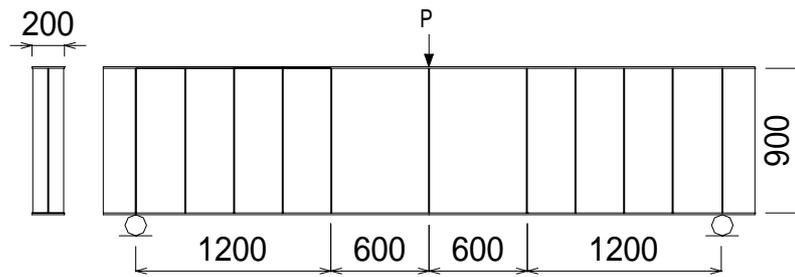
Fig.5 Bending and shear test.
