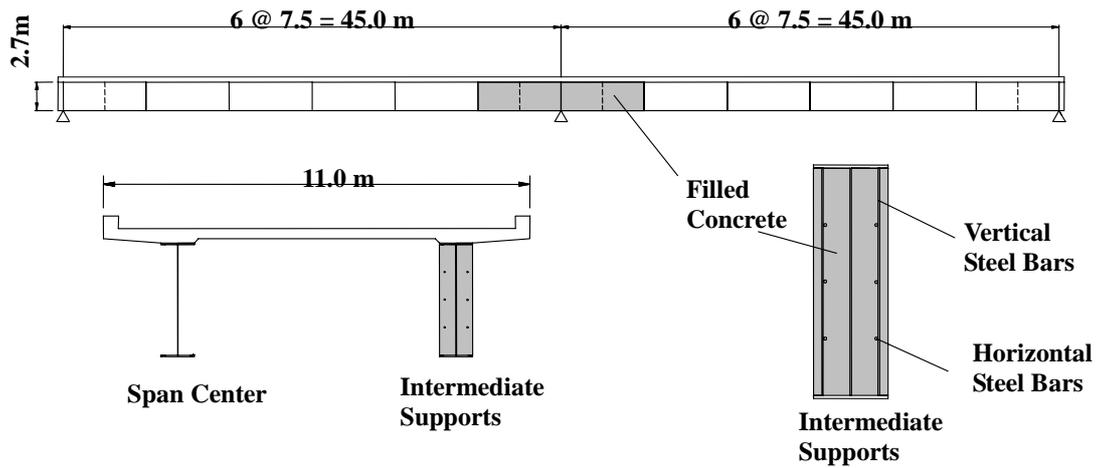
Fig.1 Partially concrete-filled steel I-girder Bridge.
