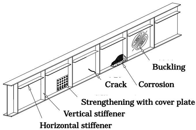
Fig.2 Damage of the steel I-girder bridge and the Strengthening(Repair).
