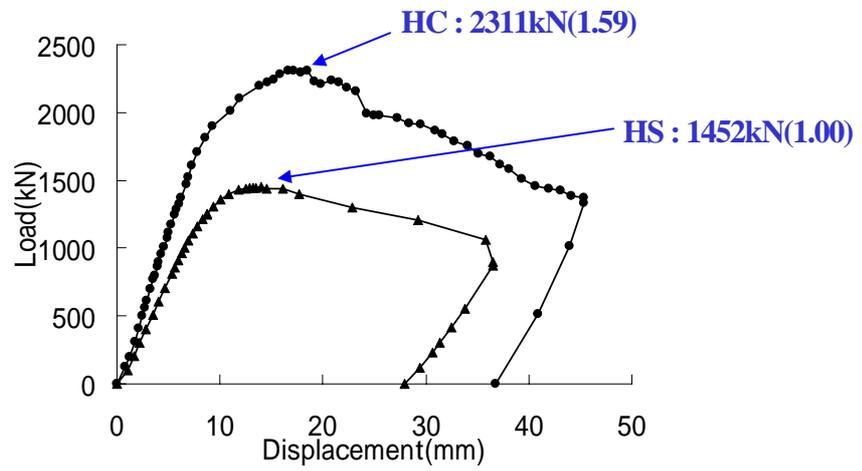
Fig.9 Load and Displacement in bending and shear test.
