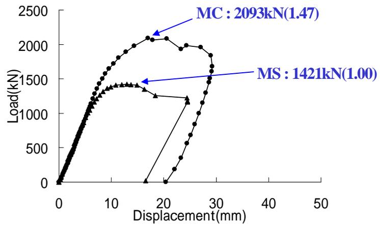
Fig.8 Load and Displacement in bending test.
