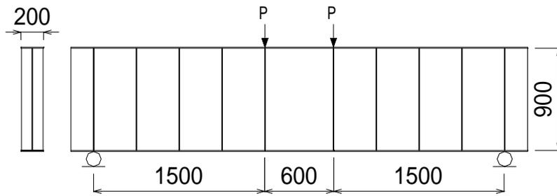
Fig.4 Bending Test.
