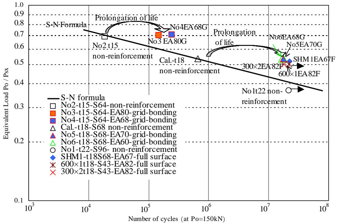
Figure 7 The relationship between number of cycles until failure and load  $P_o/P_{sx}$
