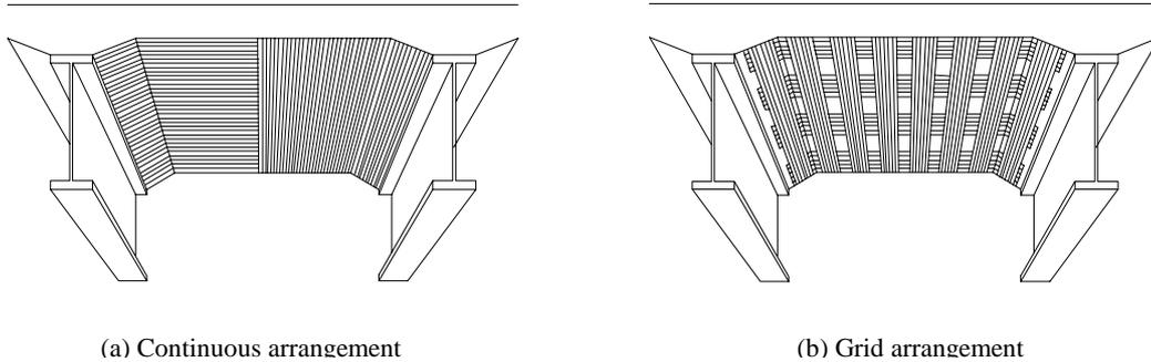
Figure 1 Arrangements of CFS
