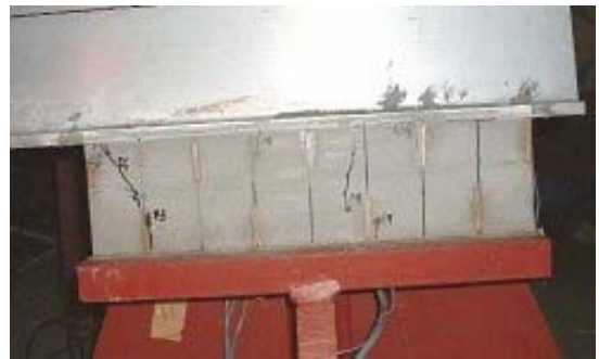
Figure10. Appearance of cracks of supporting mortar of simple beam type specimen [North connection, Back side]
