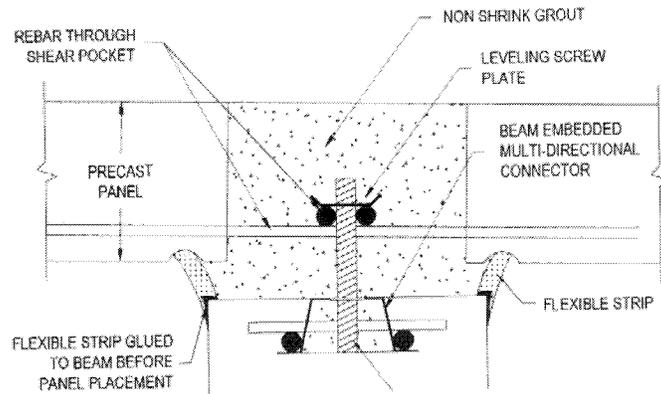
Figure 6. Grouted Shear Pocket (Source : Phelan and Vann 2004)
