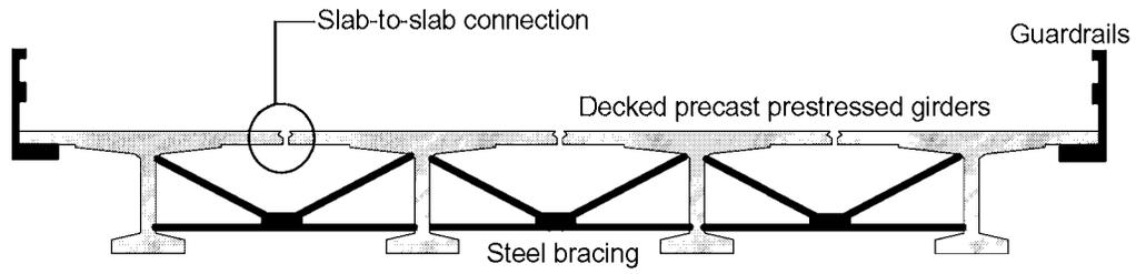
**Figure 9. Decked precast prestressed bulb-tee bridge**
