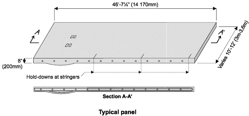
Figure 2. Prefabricated Concrete Deck Panel
