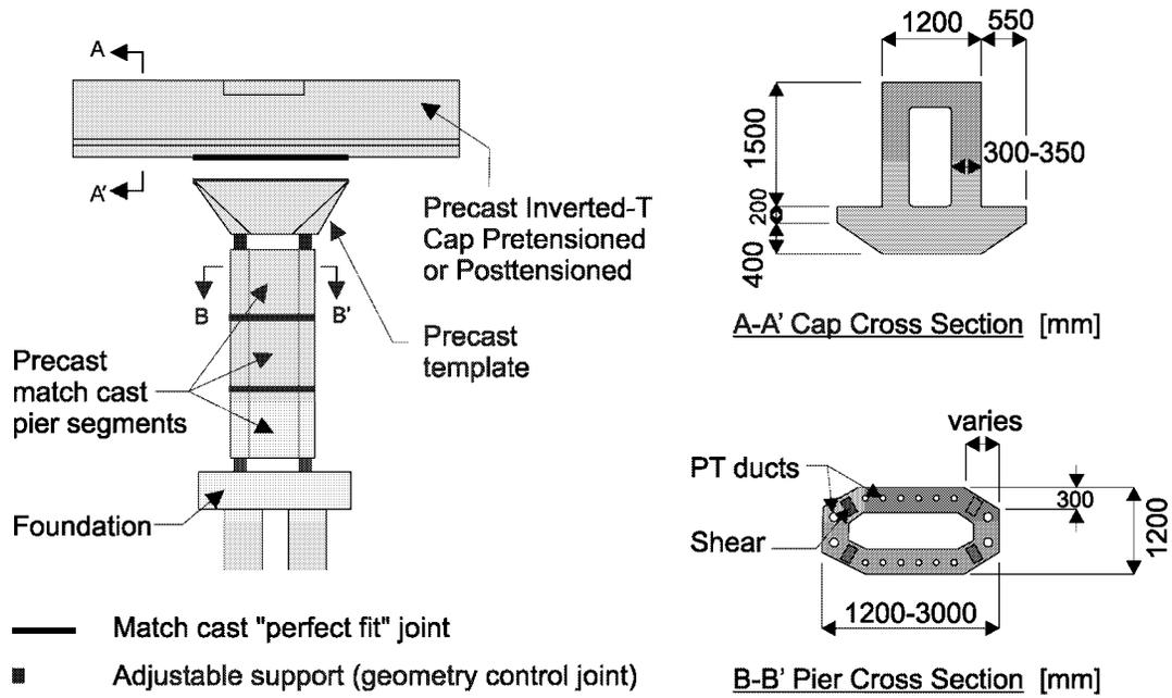
Figure 17. Segmental Pier System (Source: Billington et al. 2001)
