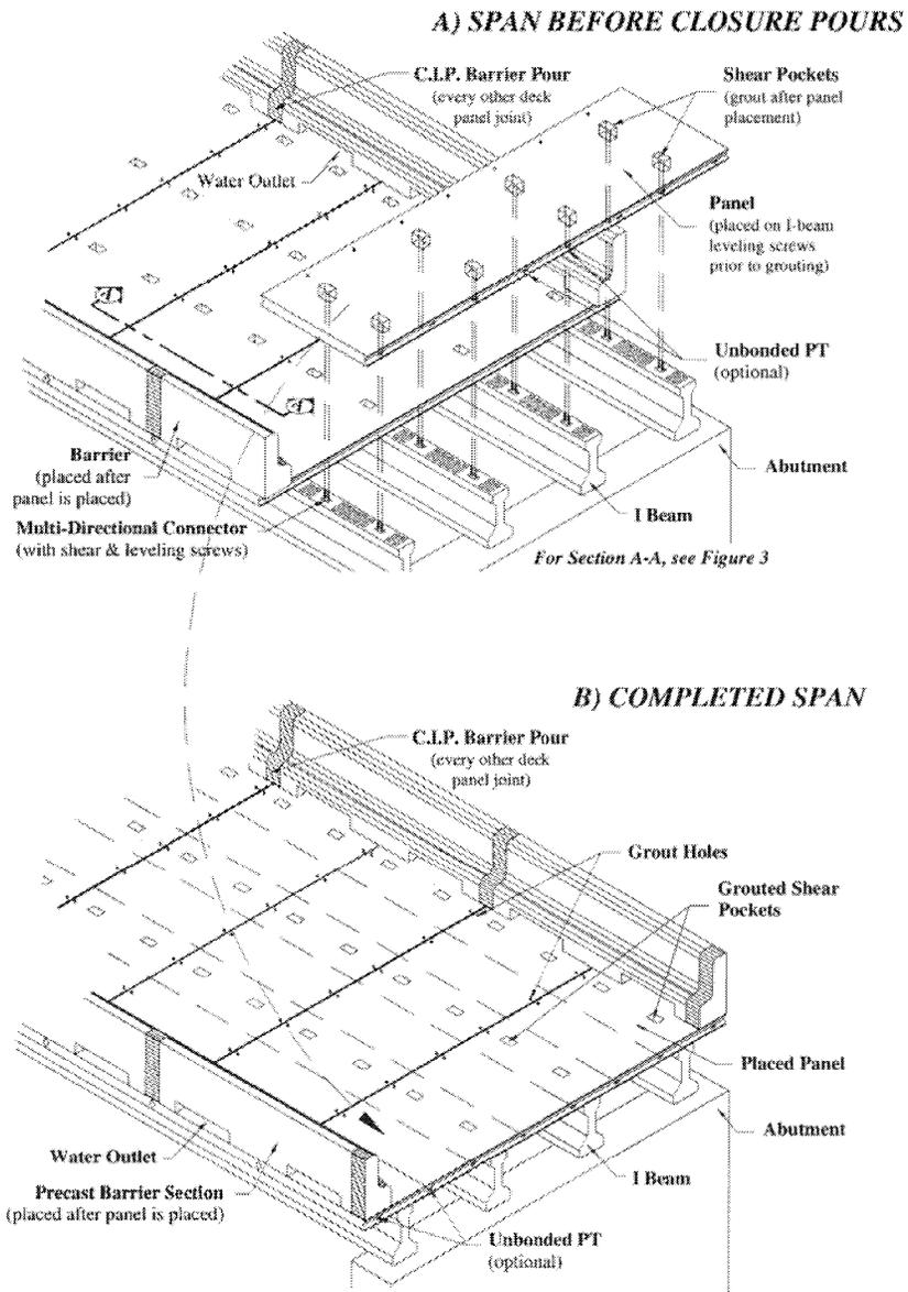
Figure 5. Superstructure System Using Full-Width, Full-Depth Prefabricated Panels
