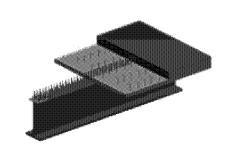
One system in Germany involved the casting of partial depth concrete decks on steel or concrete beams prior to erection of the beams. After the beams are erected, the edges of each deck unit abut the adjacent member and there is no need to place additional formwork for the cast-in-place concrete. This process speeds construction and reduces the potential danger of equipment falling onto the roadway below since a safe working surface is available immediately after beam erection.
