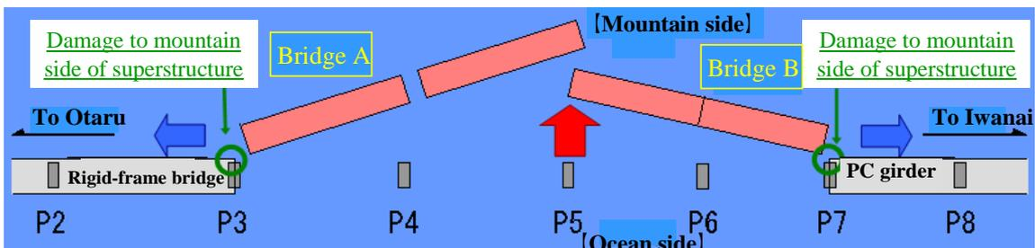
Figure 7: Postulated process of girder fall
