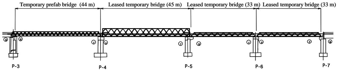
Figure 9: Side view of temporary bridges
