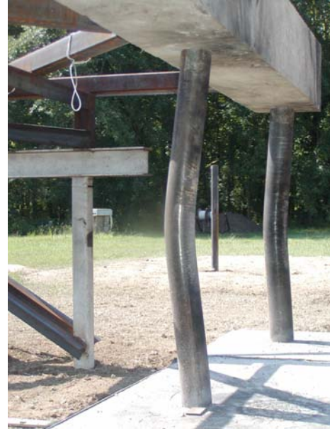
Figure 4. Bent 1-C5 (#5) after the test
