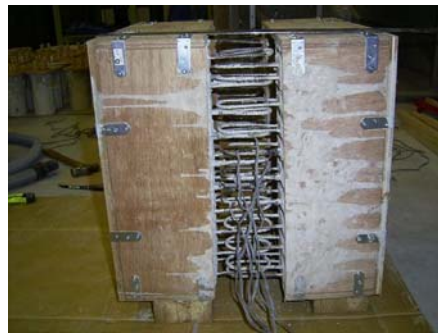
Photo.4 Assembling of loop joint
