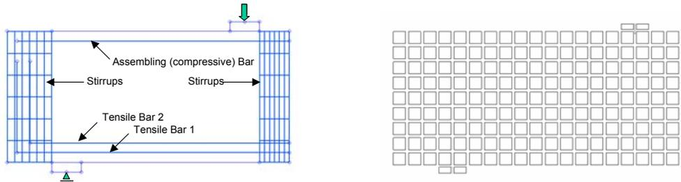
**FIG.5.** ANALYTICAL MODEL AND FE MESH DISCRETIZATION (SHRINK MESH)
