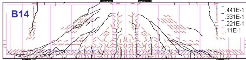
**FIG.9. B14 CRACK PATTERNS OF ANALYSIS AT ULTIMATE STATE VERSUS EXPERIMENT**
