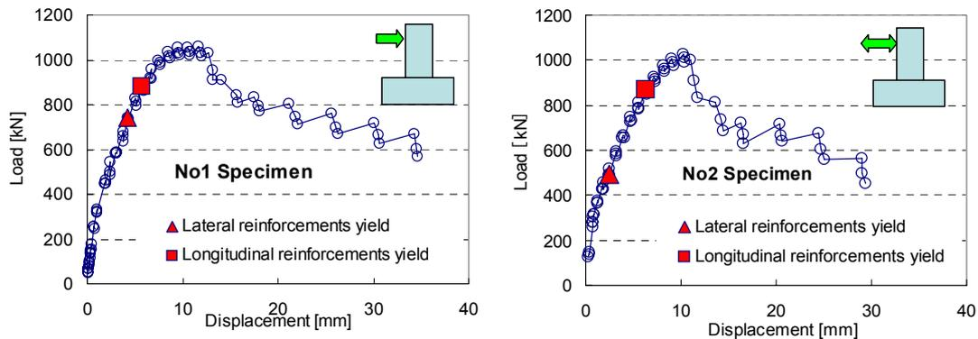
FIG.11. ENVELOPE OF CYCLIC RESPONSE OF SPECIMENS
