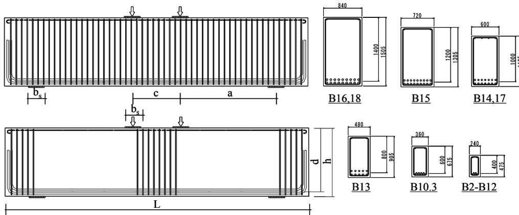
FIG.2. DETAIL OF SPECIMENS WITH AND WITHOUT STIRRUPS (UNIT: MM)
