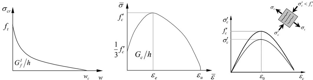
**FIG.6.** TENSILE CONCRETE MODEL **FIG.7.** COMPRESSIVE CONCRETE MODEL AND SOFTENING DUE TO LATERAL TENSILE CRACKS
