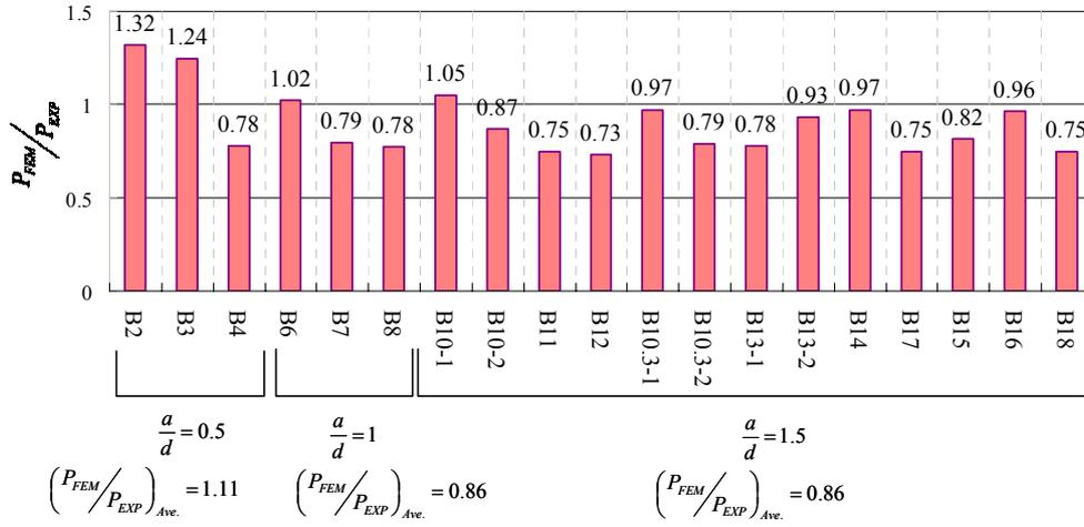
**FIG.8.** ANALYSIS VERSUS EXPERIMENT REPRESENTED BY  $P_{FEM}/P_{EXP}$  RATIO
