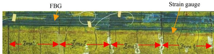
Fig.7 Crack distributions at bottom surface after experiment
