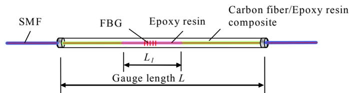
Fig.5 Special packaging for enhancing strain sensitivity
