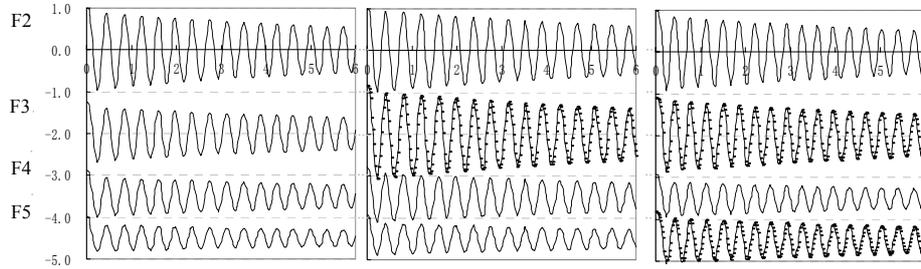
Fig.13 Macro-strain time histories of the beams from F2~F5 in S2
