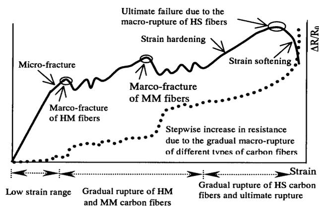
Fig.2 Electrical and mechanical models of the HCFRP sensors
