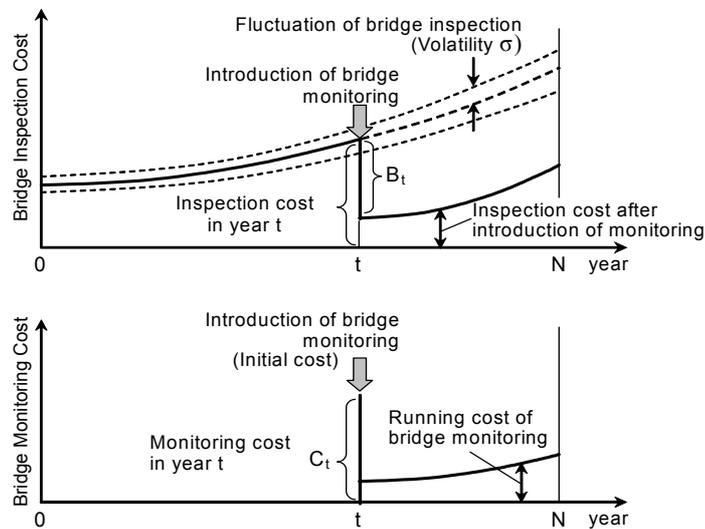
Fig.1 Modeling of bridge inspection and monitoring cost
