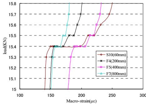
Fig.9 Crack monitoring based on strain sensors of different gauge lengths
