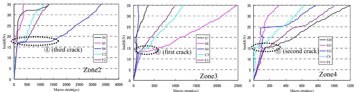
Fig.8 Crack detection with long-gauge FBG sensors
