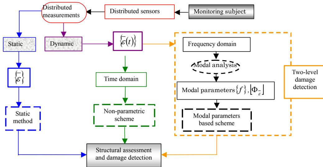
Fig.14 Structural assessment and damage detection strategy
