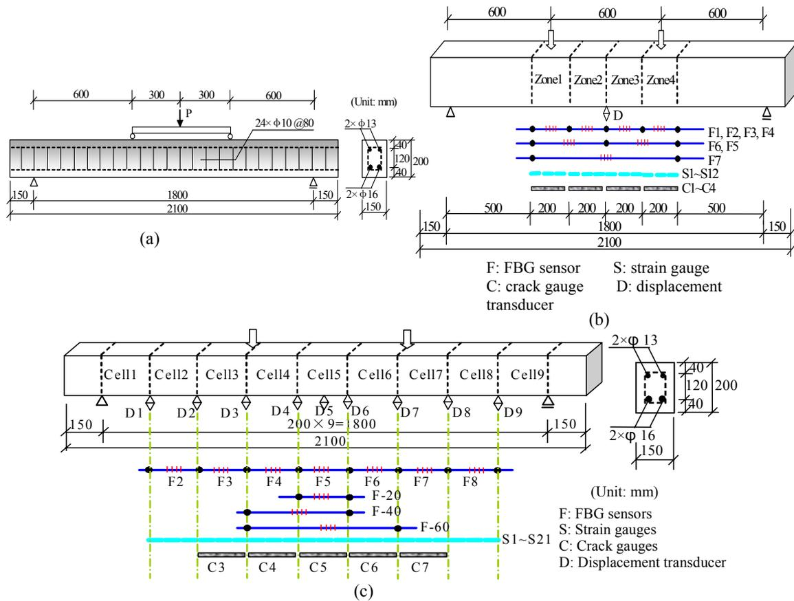
Fig.6 Outline of the RC beam: (a) dimension of the RC specimen; (b) distribution of long-gauge FBG sensors; (c) distribution of long-gauge FBG sensors with high sensitivity
