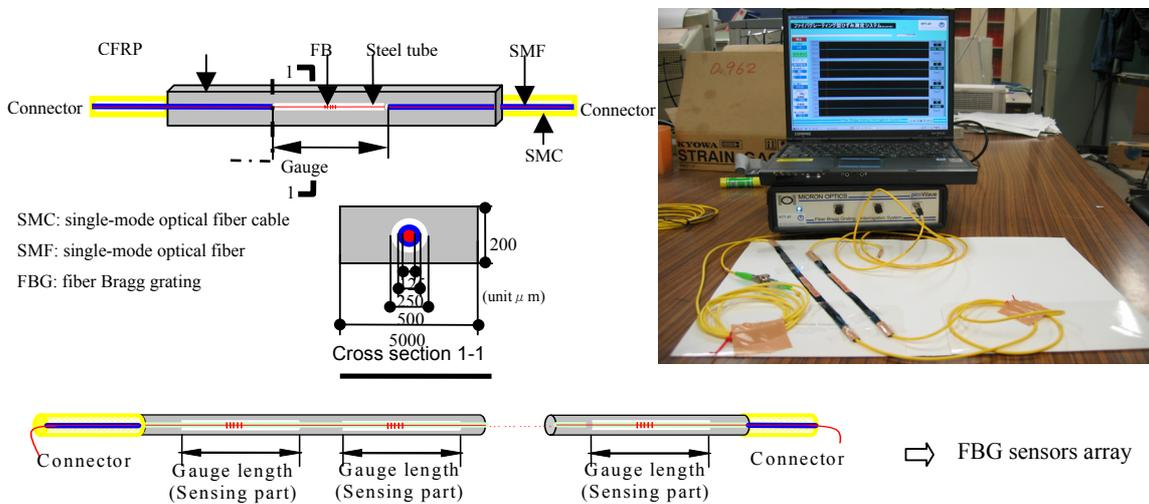
Fig.4 Developed long-gage FBG sensing system
