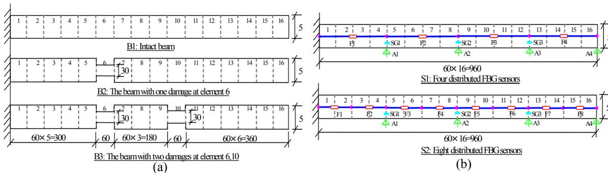
Fig.12 Experimental details about dynamic testing: (a) dimensions of specimen; (b) distribution of long-gauge FBG sensors
