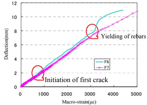
Fig.10 Deflection vs. macro-strain curves from F6 and F7
