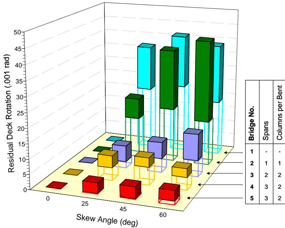
Figure 11. Range of Residual Deck Rotations
