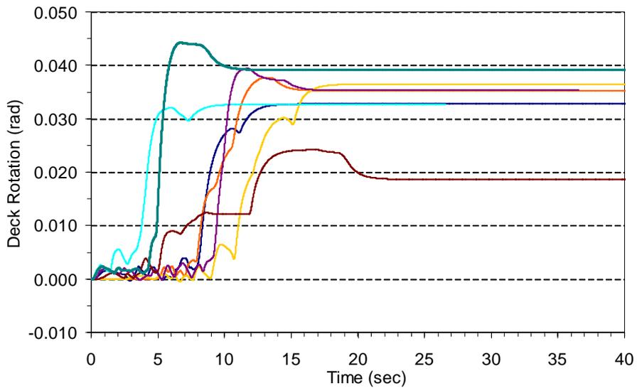
**Figure 5. Time Histories of Deck Rotation for Bridge No. 1**
