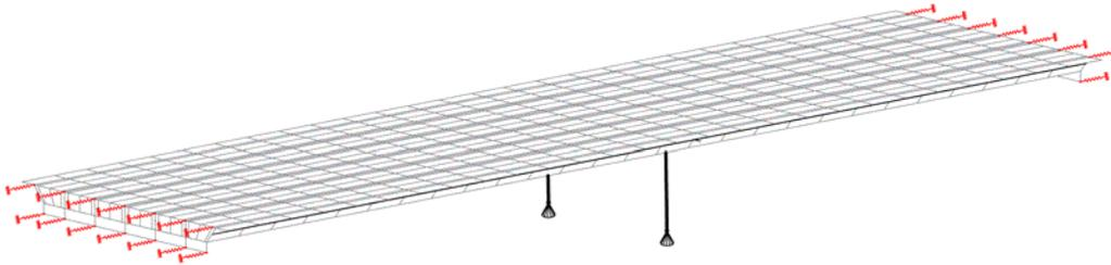
**Figure 2. Typical Bridge Model Using Shell Elements**
