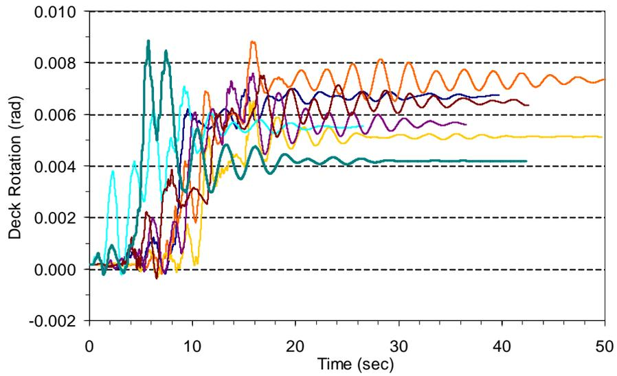
**Figure 8. Time Histories of Deck Rotation for Bridge No. 4**
