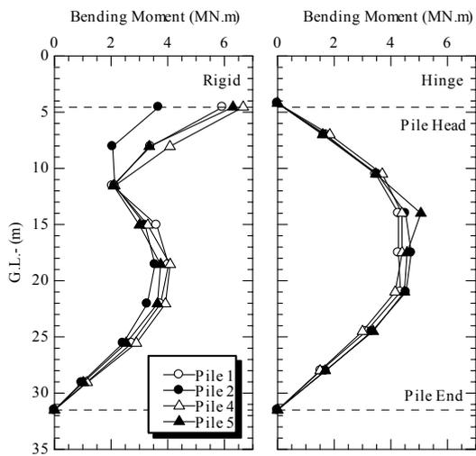
Fig.7 Maximum Bending Moment of Piles
