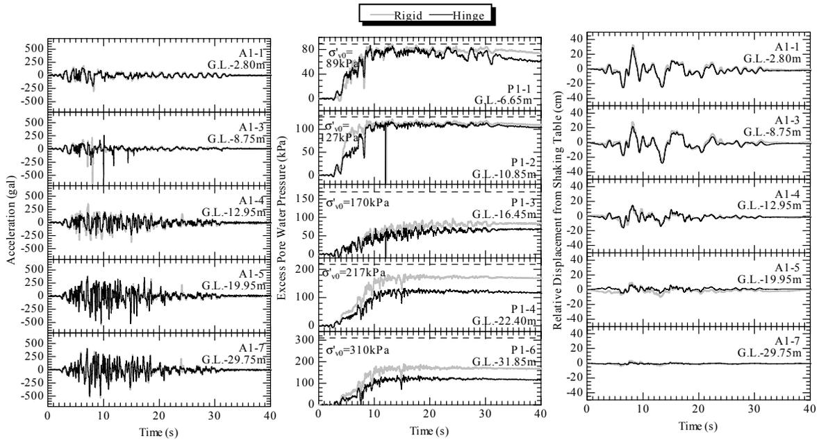
Fig.5 Acceleration, Excess Pore Water Pressure and Surface Displacement
