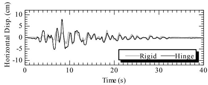
Fig.10 Relative Displacement of Footing and Ground Surface
