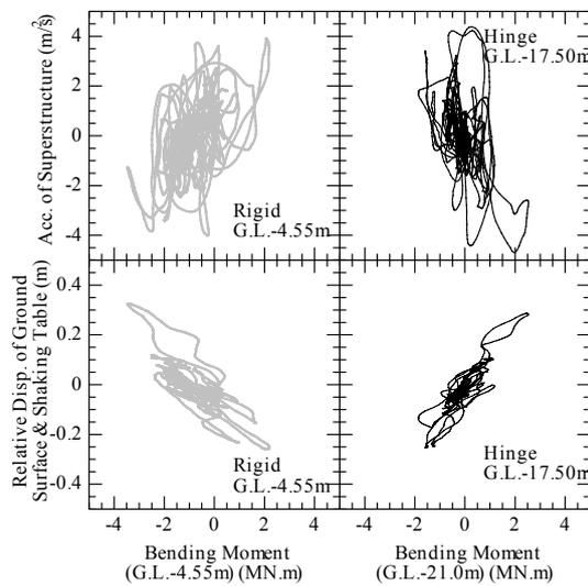
Fig.8 Phase Relationship Bending Moment ~ Ground Disp./ Pier Acc.
