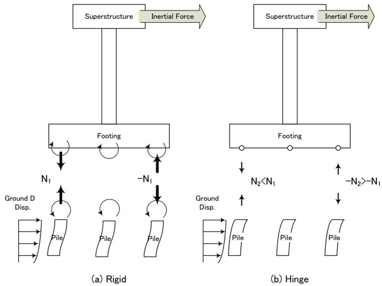
Fig.14 Variation of Sectional Force depending on Connecting Condition
