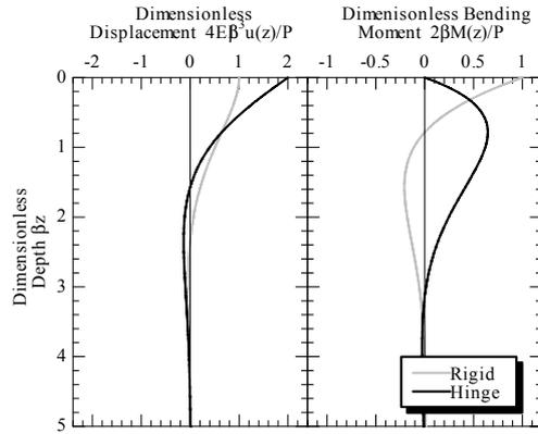
Fig.1 Analytical Solutions of Pile Displacement and Bending Moment
