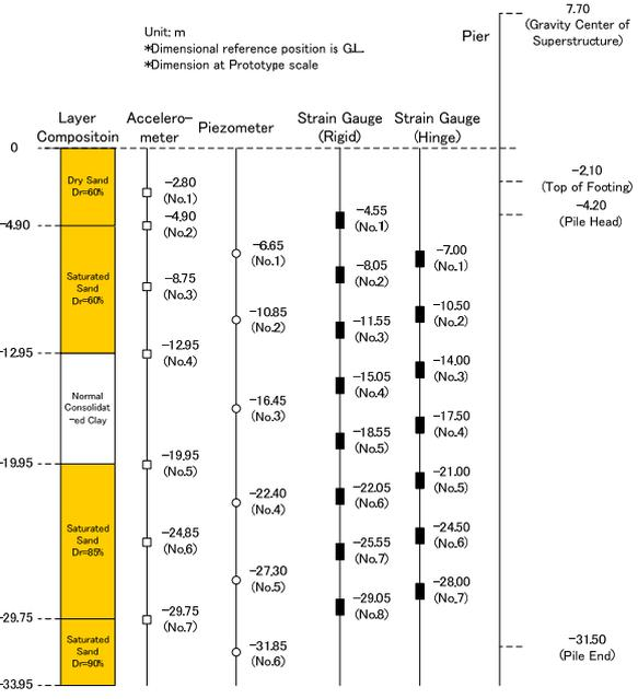
Fig.3 Sensor Configuration
