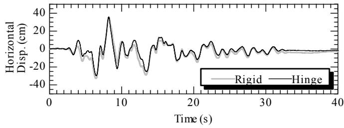
Fig.9 Relative Displacement of Footing and Shaking Table
