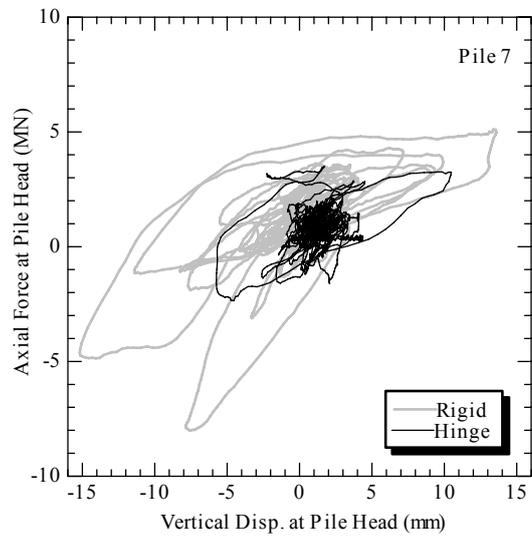
Fig.13 Relationship between Axial Force and Axial Displacement at Pile Head
