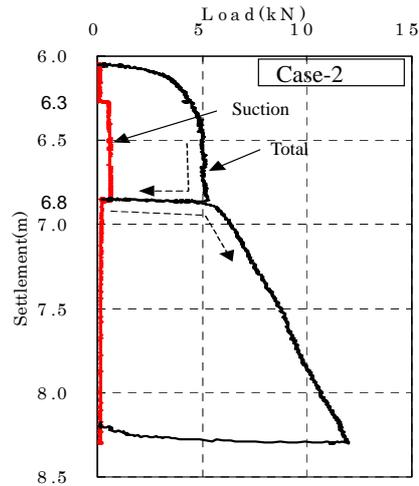
**Fig.18** Load-settlement curve of suction preloading
