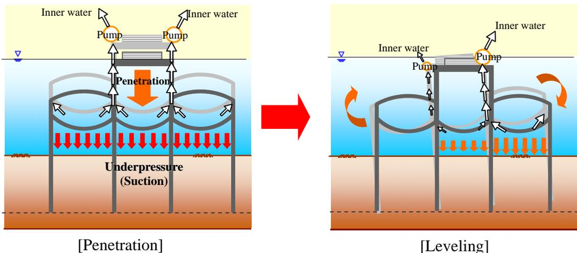
**Fig.6** Penetration and leveling of foundation due to suction
