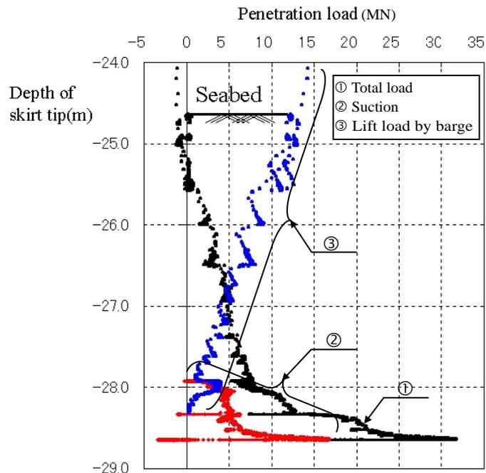
**Fig.10** Penetration load vs skirt tip depth
