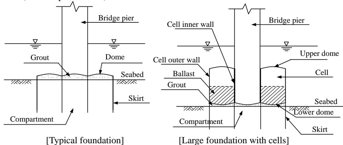
**Fig.3** Structural configuration of skirt suction foundations
