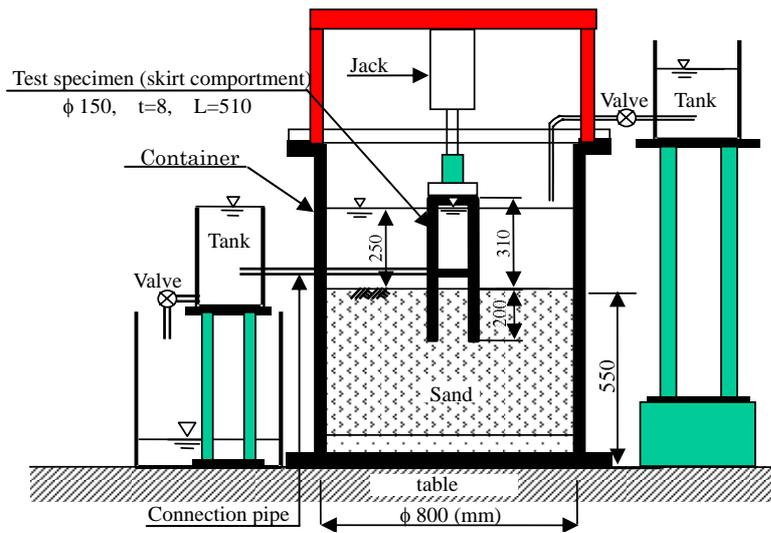
**Fig.15** Apparatus and scale model of experiment on table
