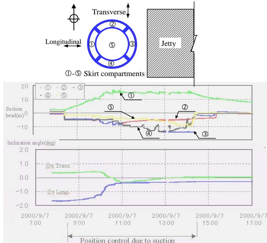
**Fig.11** Control of inclination due to suction
