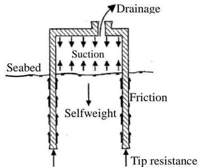
**Fig.5** Force equilibrium during suction installation
