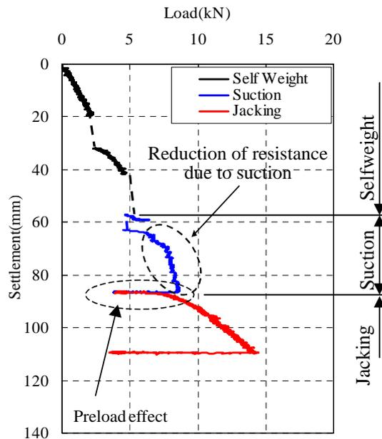
**Fig.19** Load-settlement curve of Case-3
