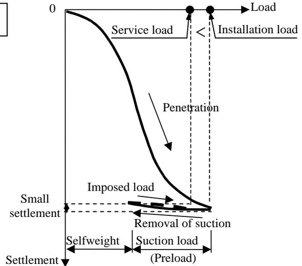
**Fig. 13** Schematic description of preload effect
