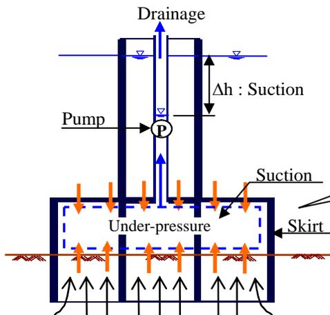
**Fig.4** Seepage during suction installation
