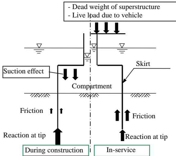
**Fig. 12** Concept of "Preload" due to suction
