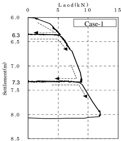
**Fig.17** Load-settlement curve of jack preloading
