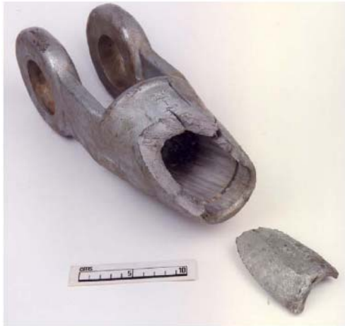
Wire Rope Socket Premature Failure
