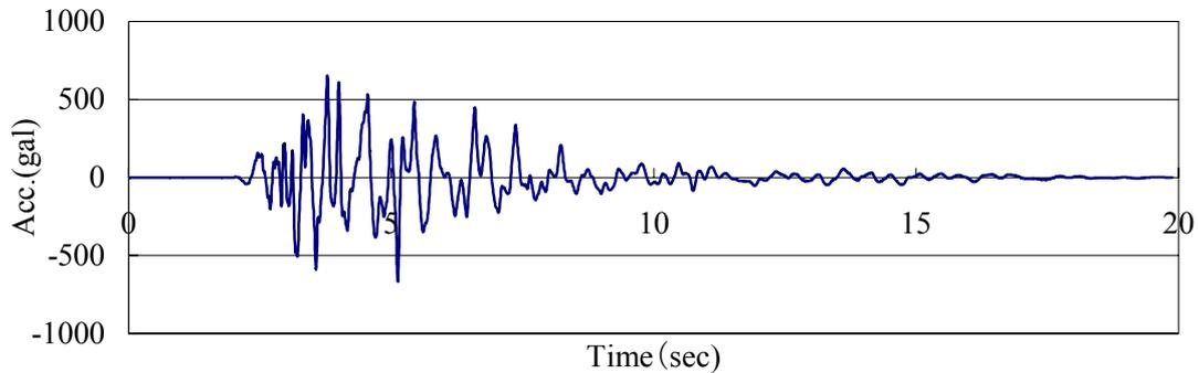
**Fig.4 Input waveform (The scaling factor of time is 1/ 5)**
