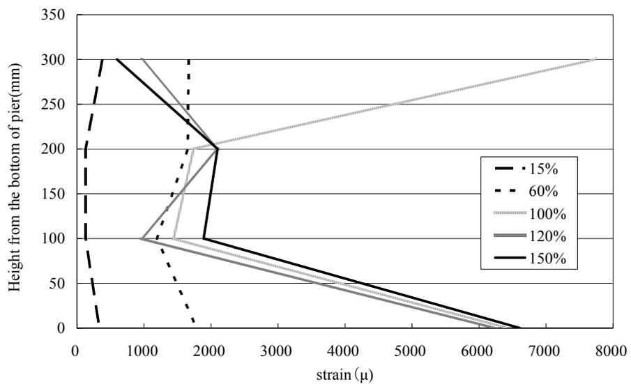
**Fig.5 Distribution of longitudinal reinforcement strain**
