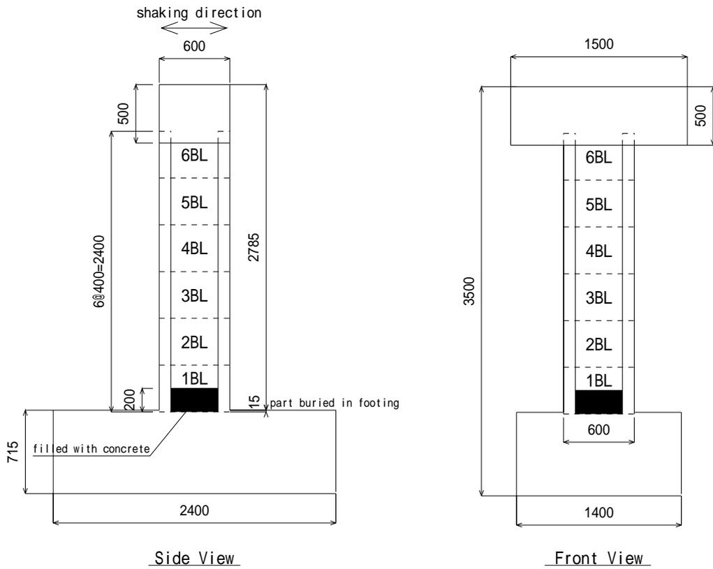
**Fig.1 Specimen Views (unit: mm)**
