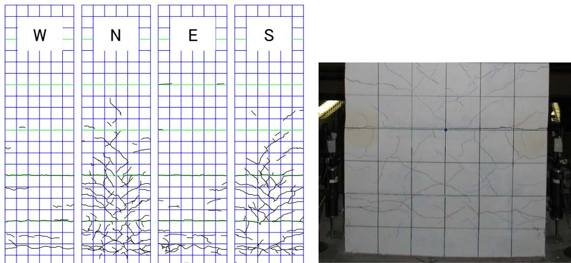
**Fig.7 Damage after Case5 (150%)**
