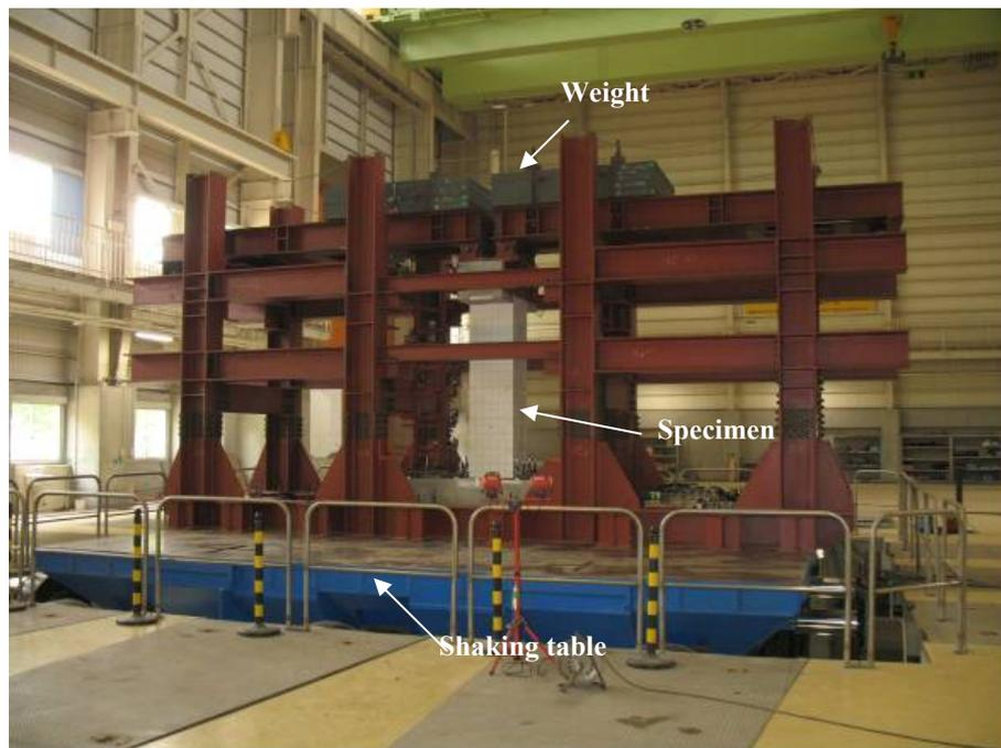
**Fig.3 Test Setup**
