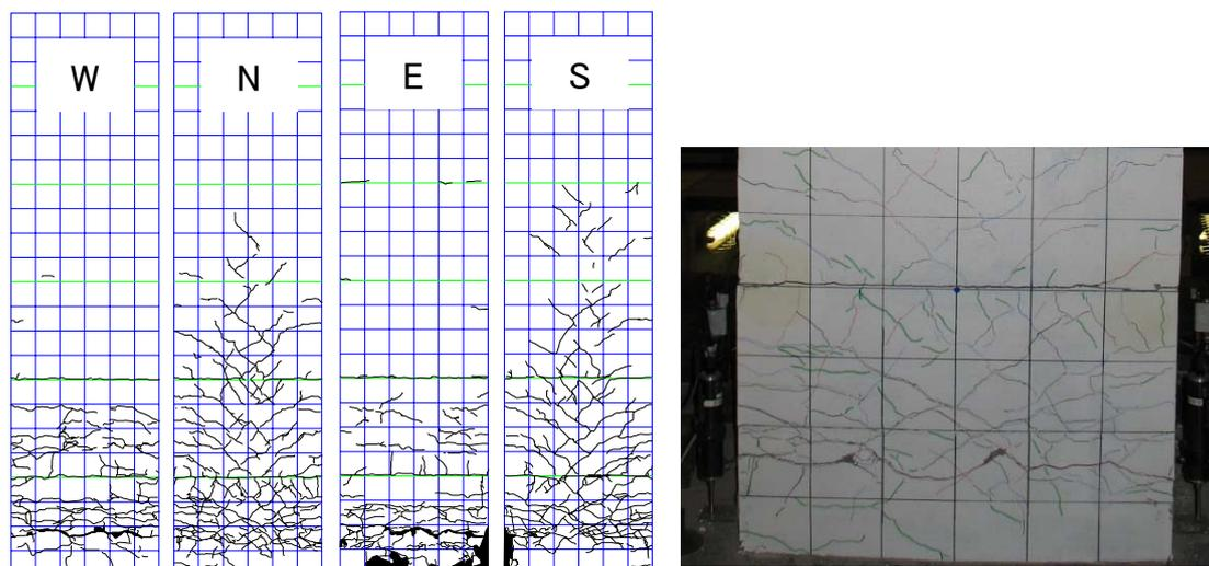
**Fig.8 Damage after Case7 (250%)**
