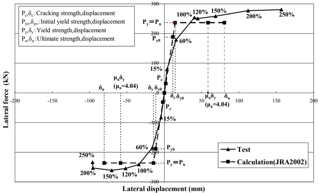
**Fig.10 Lateral force vs. lateral displacement**
