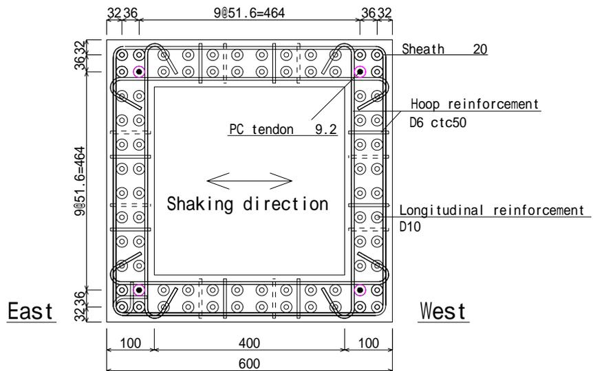
**Fig.2 Specimen Cross Section (unit: mm)**
