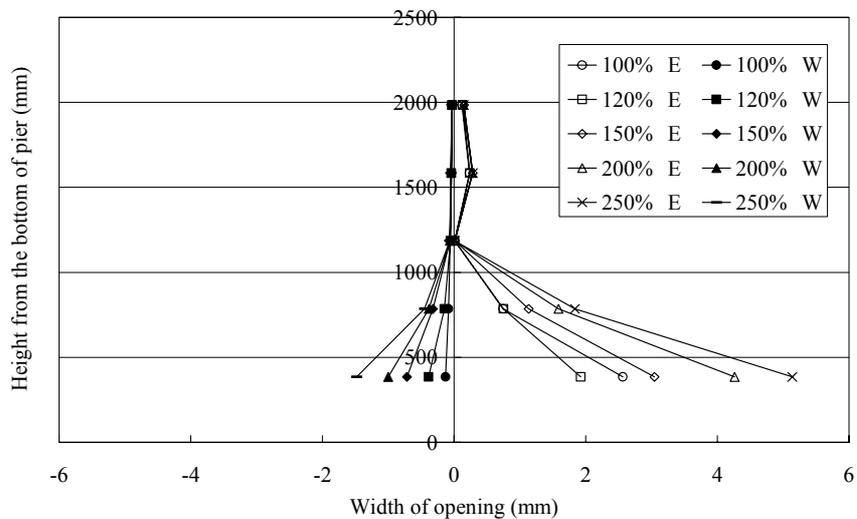
**Fig.6 Width of joint opening between segments**
