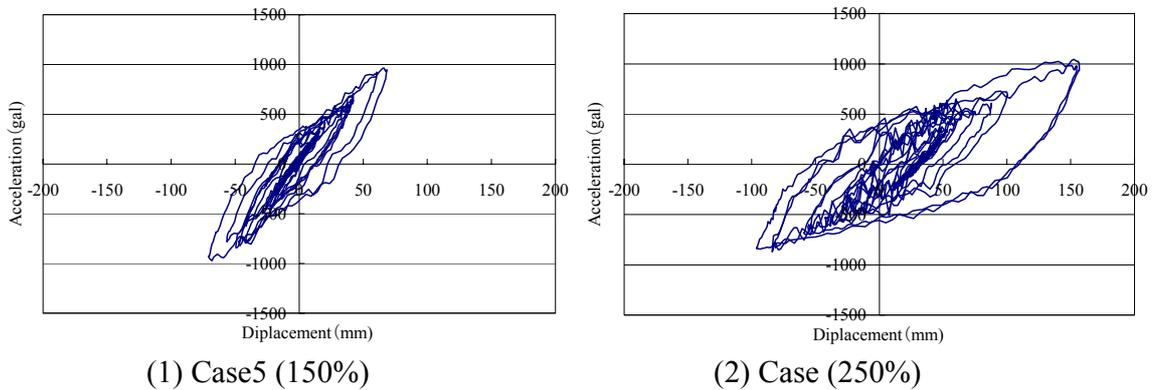
**Fig.9 Acceleration vs. displacement at the top of pier hysteresis**
