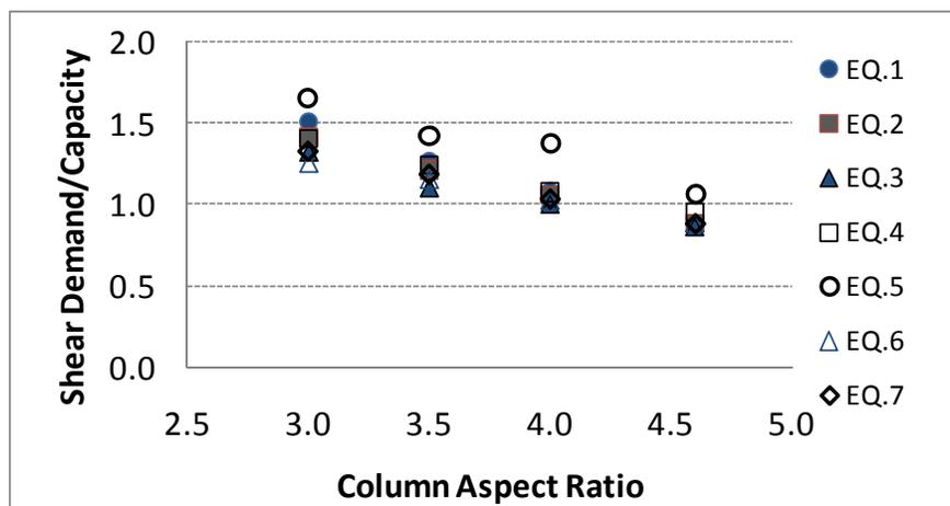
Figure 9 – Effect of aspect ratio (column height/diameter) on shear DCR
