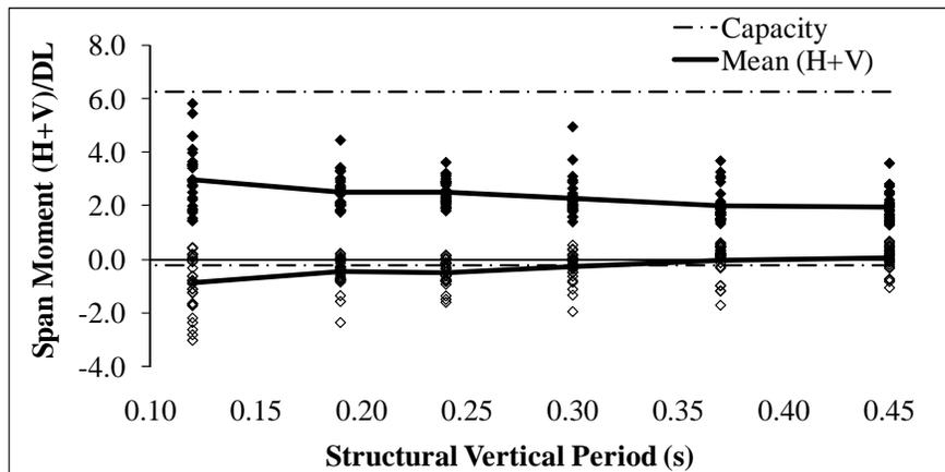
Figure 5 - Variation of moment demand at the mid-span with vertical period for unscaled ground motions
