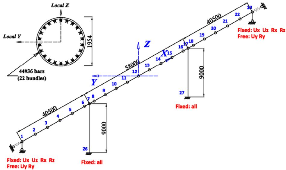
Figure 6 – Simulation model of the Plumas Bridge used in Phase II Study
