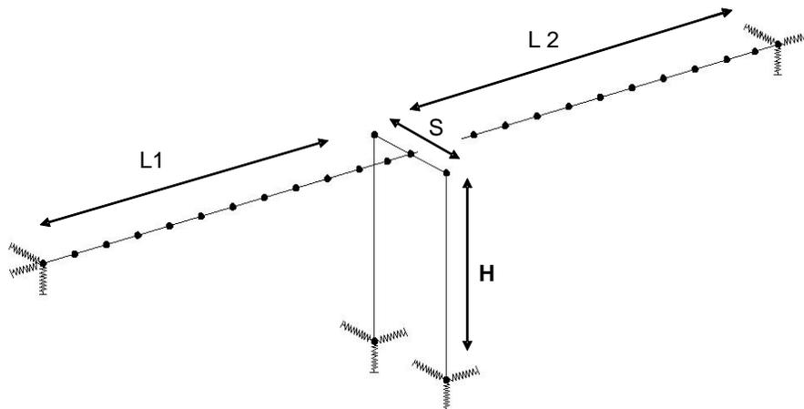
Figure 2 – Simulation model of typical two-span bridge
