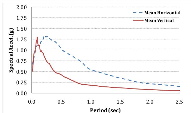
Figure 3 –Spectra of the horizontal component of ground motions scaled to match the ARS curve (Magnitude 8.0, PGA 0.5 g and site class D) at fundamental longitudinal period of base configuration, and corresponding vertical spectra
