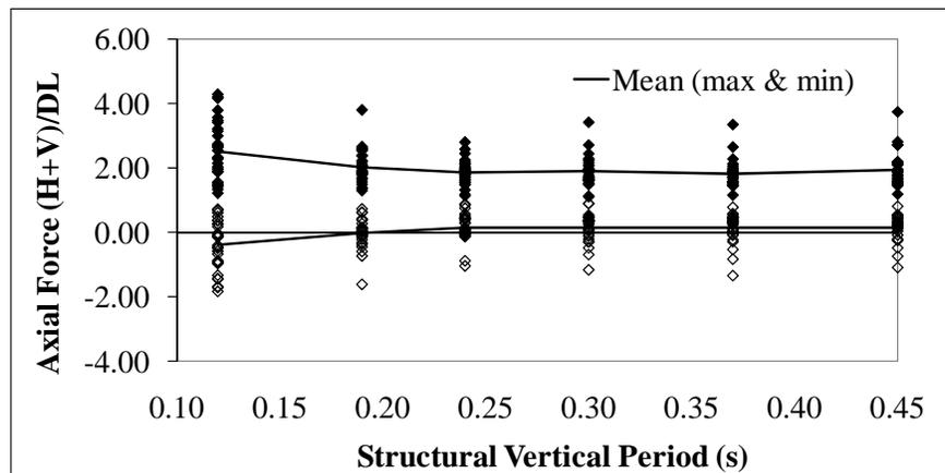
Figure 4 – Variation of column axial force demands with vertical period for unscaled ground motions
