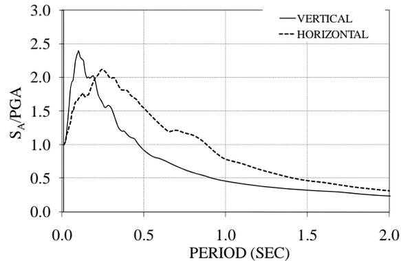
Figure 1: Characteristics of near-fault horizontal and vertical motions
