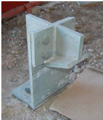
Photo 6 Device for constraint of I girders
