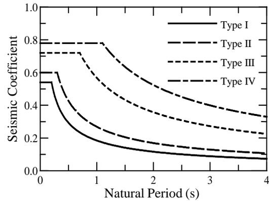
Fig. 2 Seismic coefficient by Eq. (1) assuming  $A_0=0.4g$  and  $c_I=1.0$
