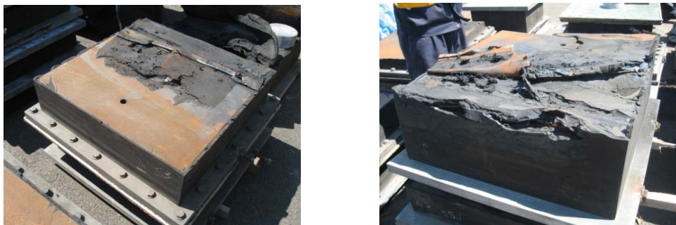
Photo 6 Details of Rupture of Elastomeric Rubber Bearings
