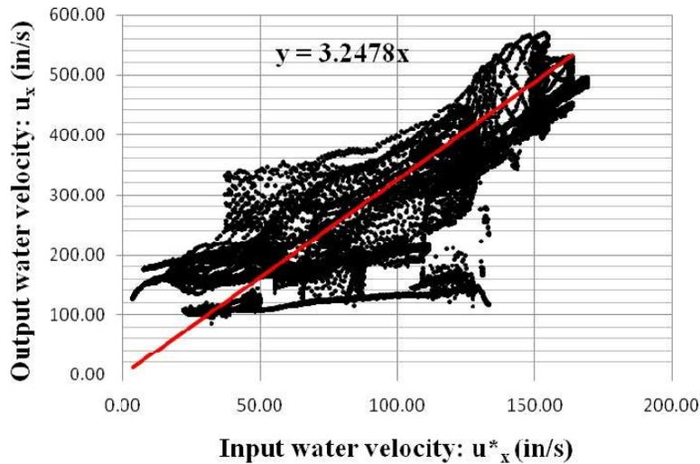
FIGURE 8, COMPARISON OF HORIZONTAL WATER VELOCITY WITH AND WITHOUT OBSTRUCTIONS (BRIDGE SUPERSTRUCTURE)
