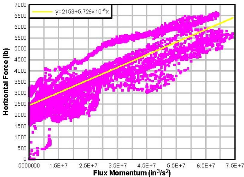
FIGURE 6, TOTAL HORIZONTAL FLUX VERSUS FLUX MOMENTUM
