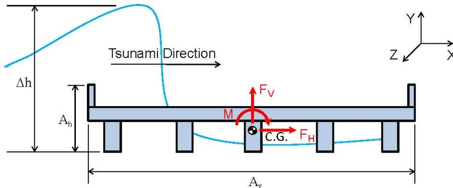
FIGURE 5, SIMULATED HORIZONTAL AND VERTICAL TSUNAMI FORCES
