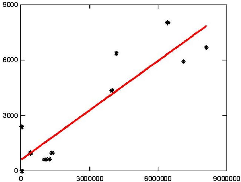
FIGURE 4, MAXIMUM FLUX (Horizontal axis,  $\text{in}^3/\text{sec}^2$ ) VERSUS MAXIMUM HORIZONTAL TSUNAMI FORCE (Vertical axis, pounds/in)
