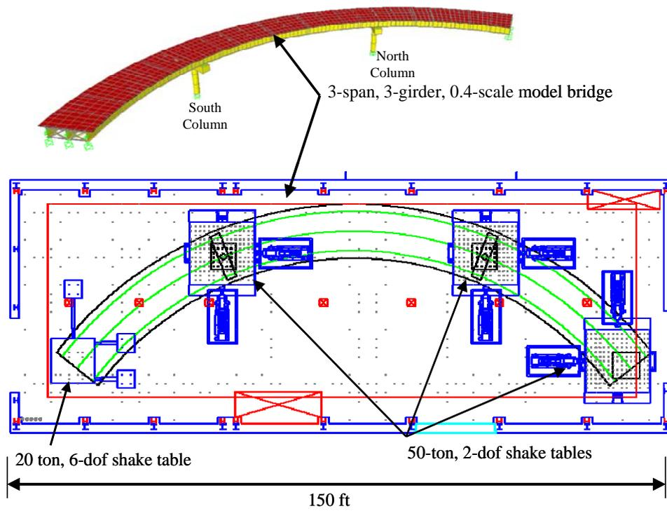
**Figure 1. Bridge Model and Layout in Large-Scale Structures Laboratory.**
