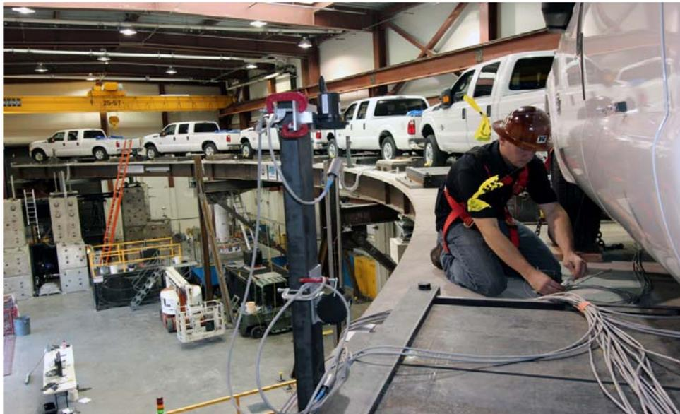
**Figure 4. Bridge Model with Live Load (Courtesy of M. Wolterbeek, 2011)**
