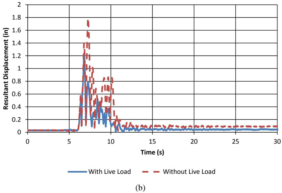
**Figure 5. (a) North and (b) South Column Displacements during 75% DE Run.**
