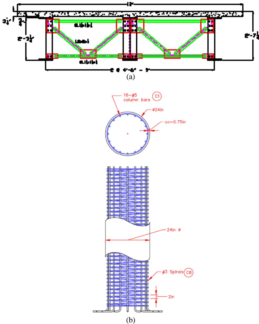
**Figure 3. Typical Superstructure and Column Details.**
