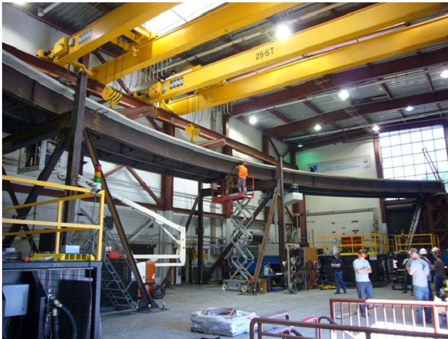
**Figure 2. Bridge Model Assembled in Large-Scale Structures Laboratory.**
