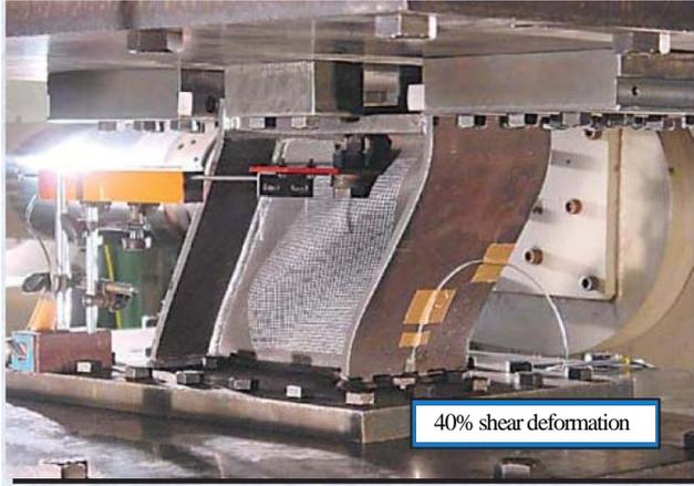
Picture 5 Shear panel damper
