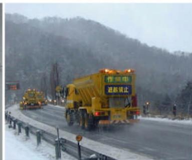
Fig.3 Scattering of deicing salts
