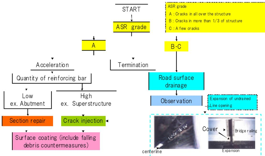
Fig.12 Selection of ASR Maintenance Method
