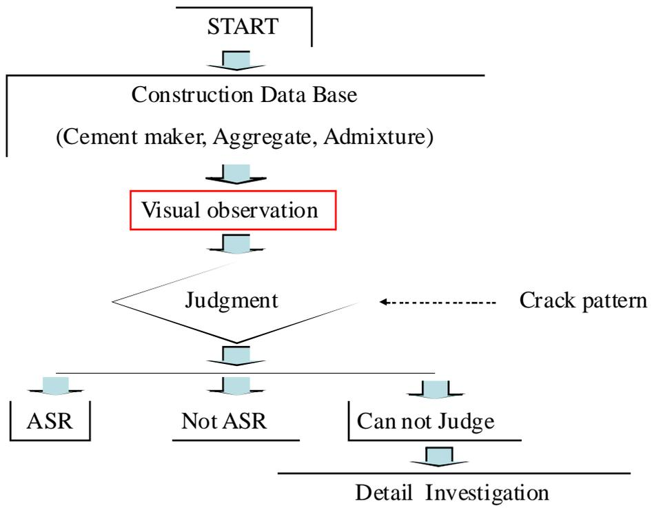
Fig.7 Flow of Assessment of ASR Structures
