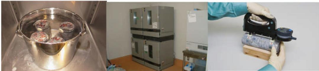
Fig.11 Residual expansion test of concrete cores
