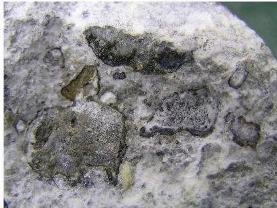
Fig.5 ASR gel (Core fracture surface)
