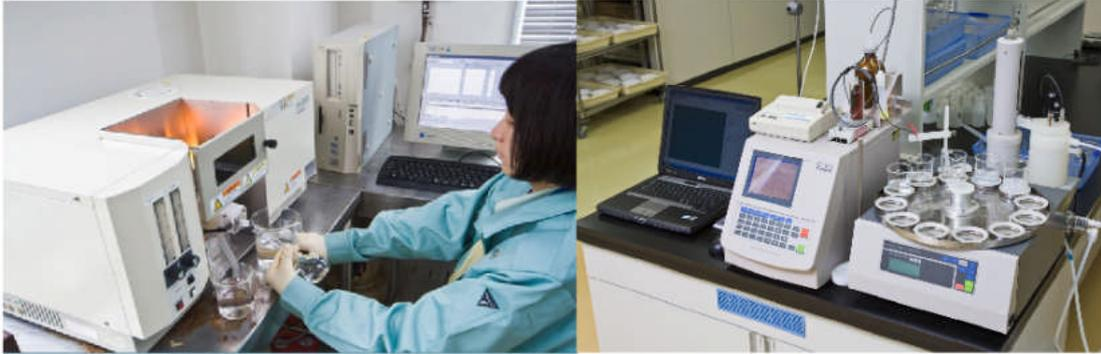
Fig.9 Alkali content of concrete by Atomic Absorption Spectroscopy Apparatus
