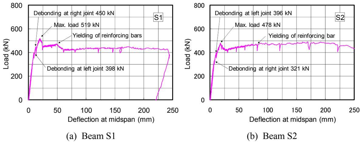
Fig. 13 Relationship between load and deflection at midspan of the old beams
