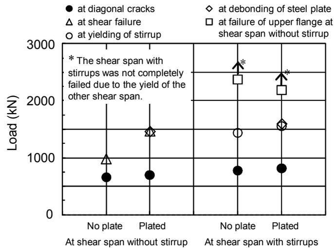
Fig. 11 Comparisons of the load at diagonal cracking, the load at debonding, and the maximum load in Series II
