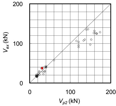
Fig. 5 Comparison between the measured shear forces at cracking at the edge of steel plate and the calculated shear force at debonding of steel plate
