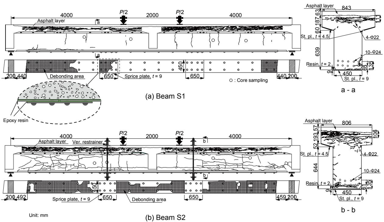
Fig. 12 Deterioration of old reinforced concrete beams with bonded steel plates
