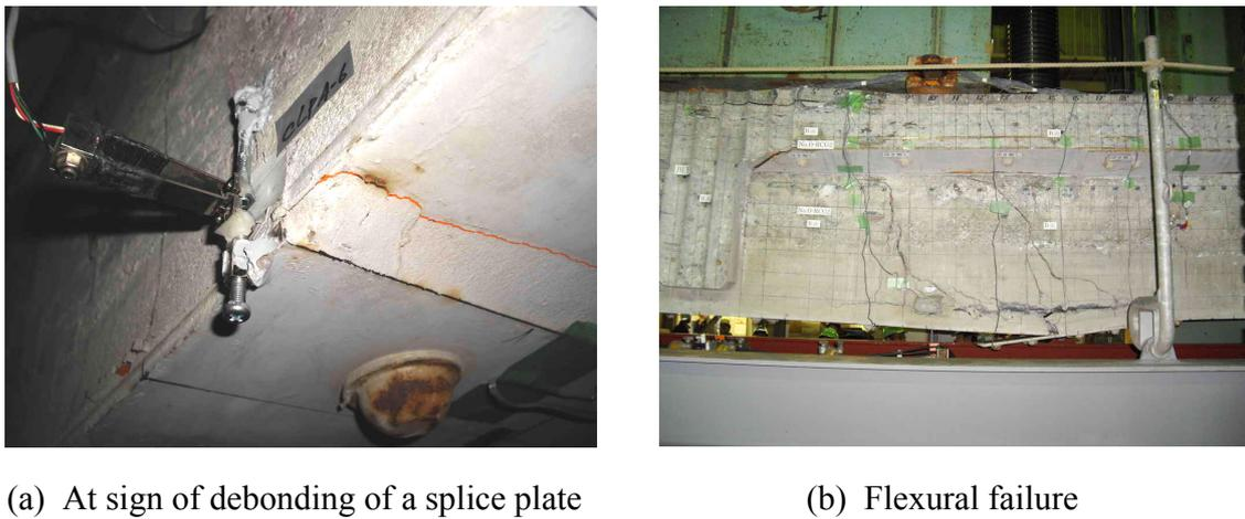
Fig. 14 Failure observed in Beam S1
