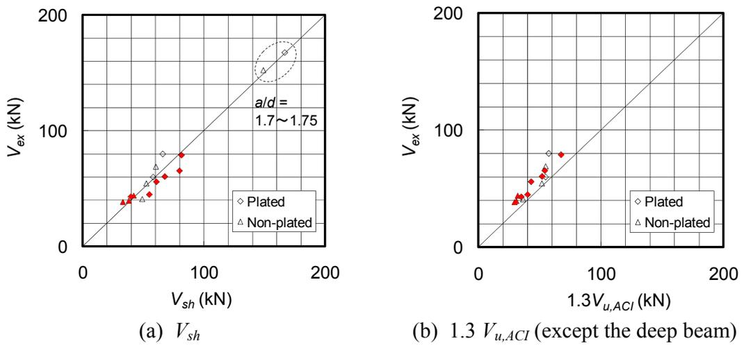
Fig. 6 Comparisons between the measured shear force of the plated beams at diagonal cracking and the calculated shear capacity for flexure-shear cracking.
