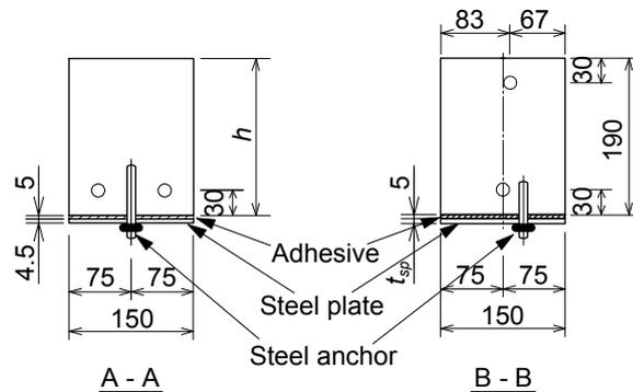
Fig. 3 Configurations of specimens in Series I
