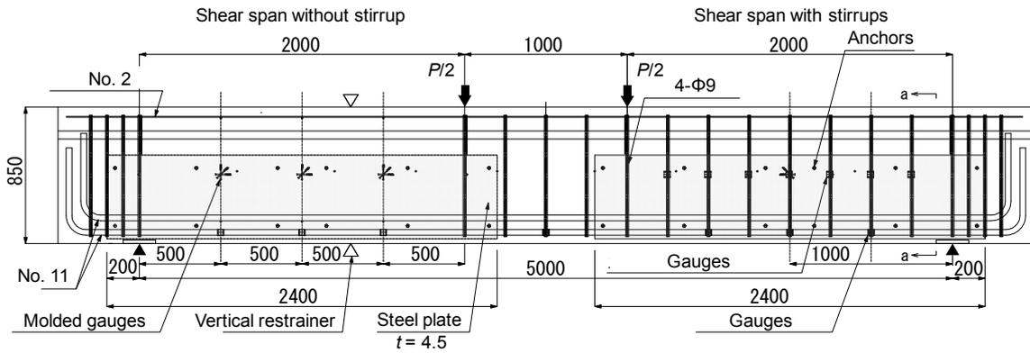
Fig. 8 Details and test setup of side-plated beams in Series II
