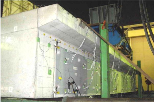
Fig. 7 Wing-type steel plates bonded to the sides of web in Series II
