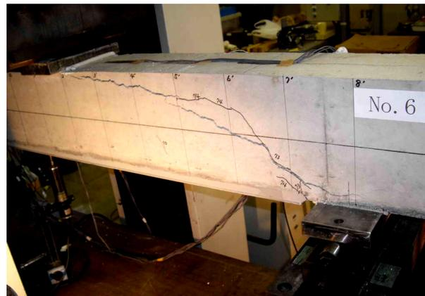
Fig. 4 Failure due to cracking at the edge of the bonded steel plate in Specimen A-6
