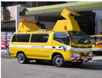
FIGURE 2 - HDV-EQUIPPED INSPECTION VEHICLE (LEFT)
