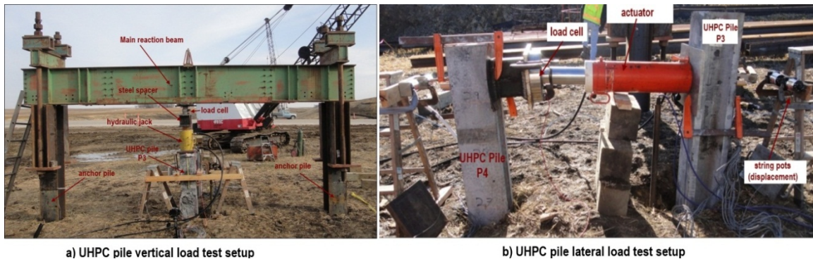
FIGURE 12: SETUPS USED FOR UHPC PILE TESTS IN THE FIELD
