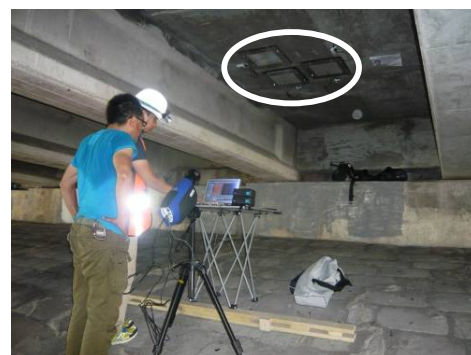
(b) TEST PIECE UNDER THE DECK
