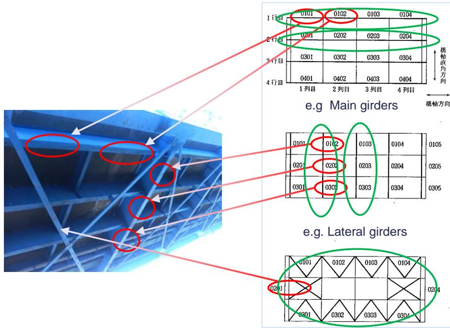
Fig. 3 Concept of unit-level BMS
