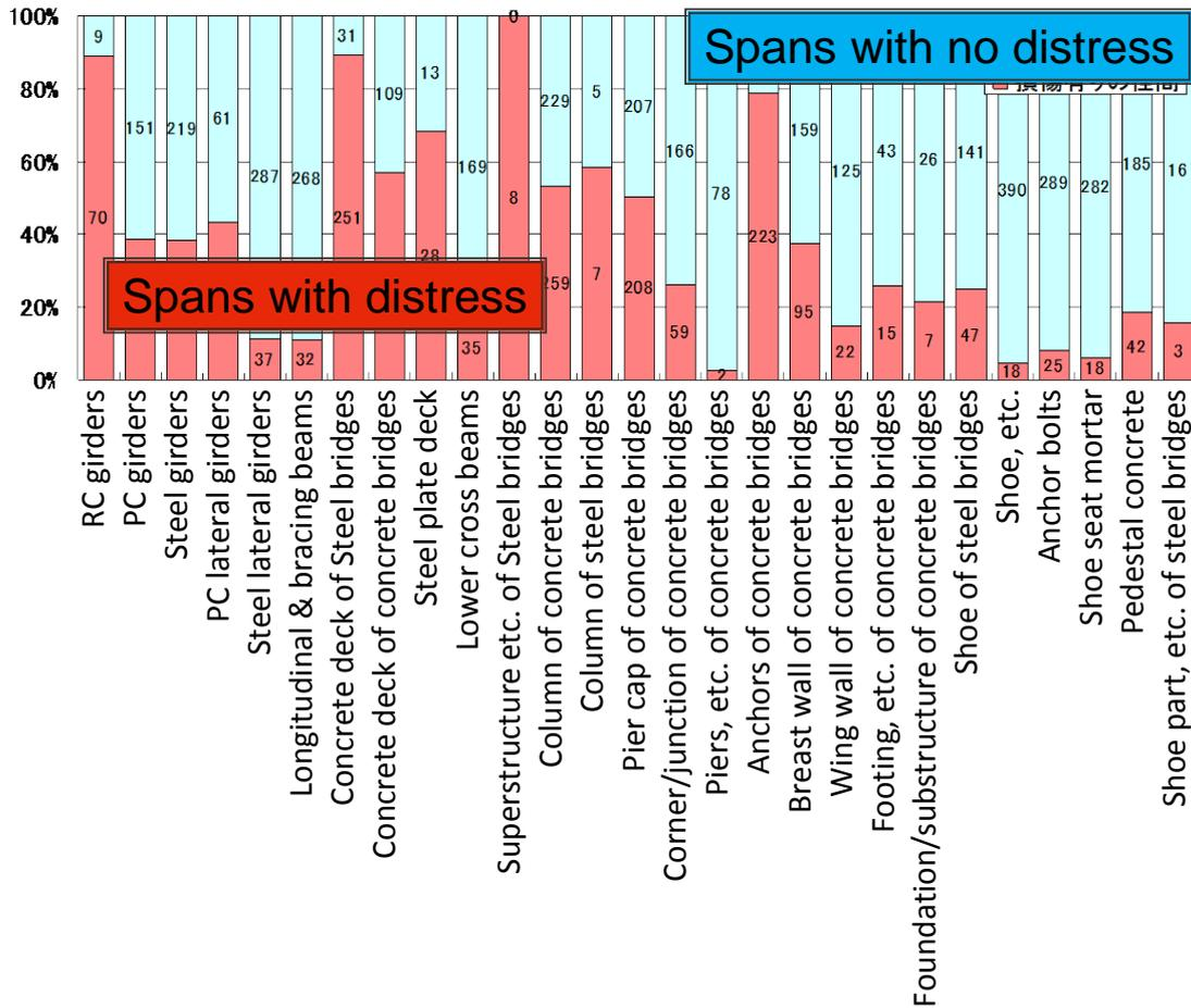
Fig. 16 Percentages of spans with and without distress
