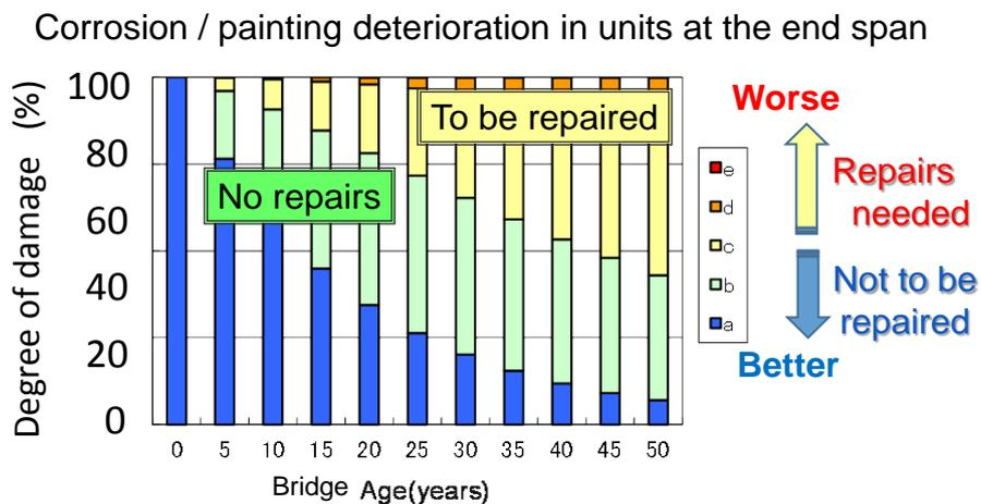
Fig. 9 Example of deterioration curves calculated by using the Markov transition probability
