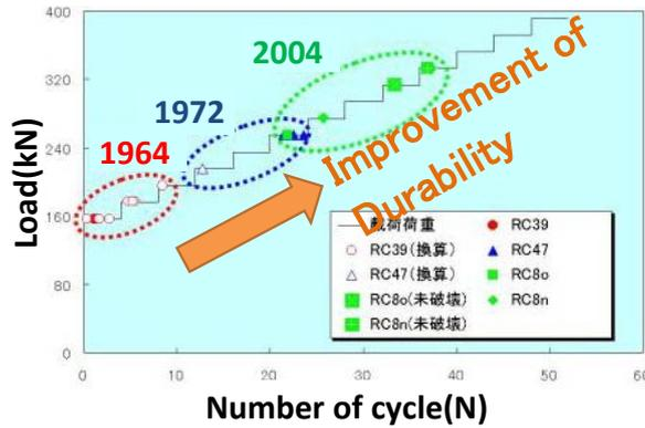
Fig. 15 Example of changes in concrete slab standards and changes in durability
