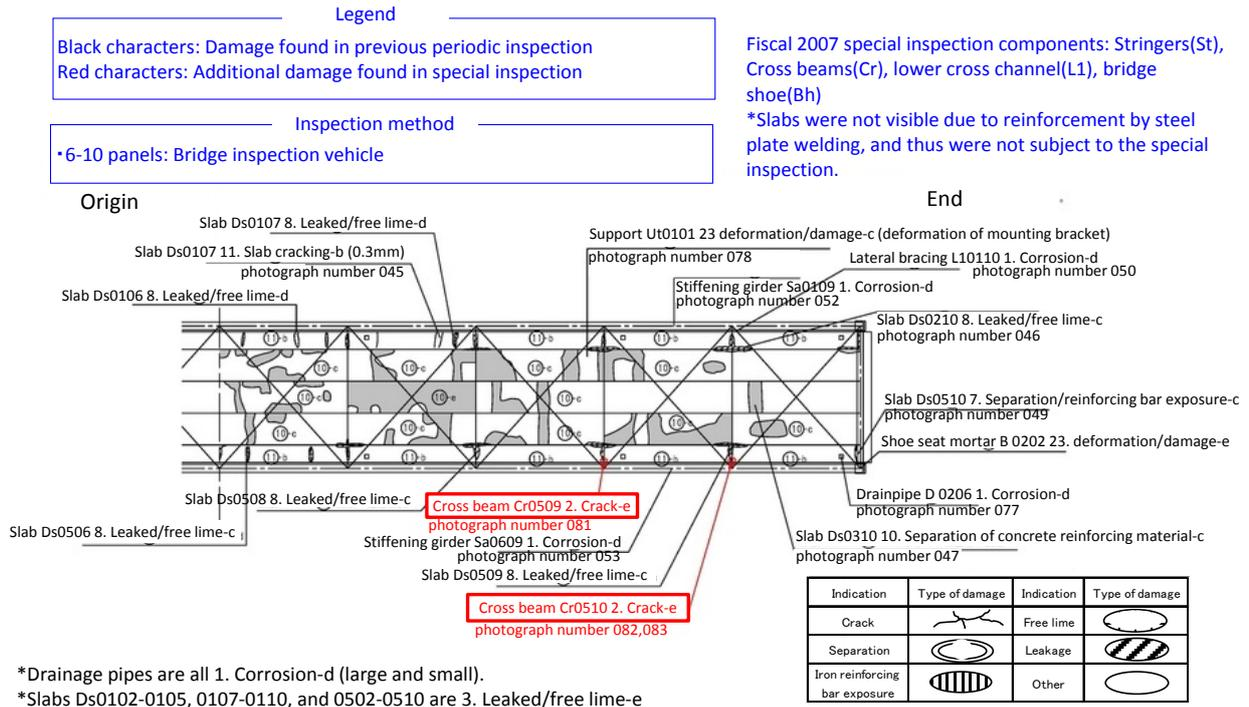
Fig. 5 Example periodic inspection record (sketch of bottom surface of deck)
