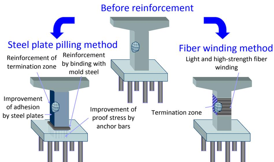
Fig. 14 Example of earthquake reinforcements
