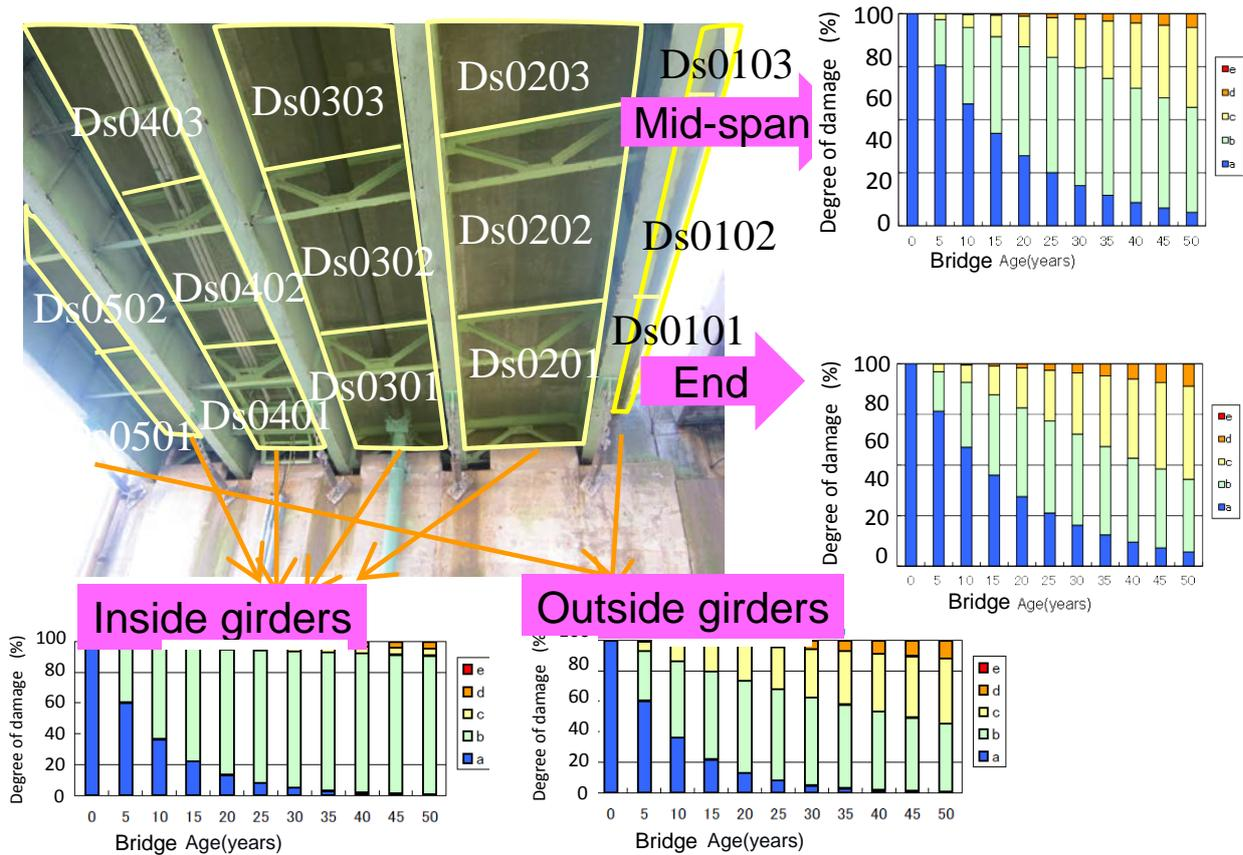
Fig. 10 Creation of deterioration curves for each element
