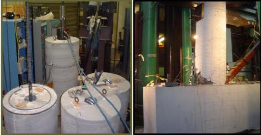
Fig. 7: Test Setups of Large Bar-duct Pullout and Column-to-cap beam Connection
