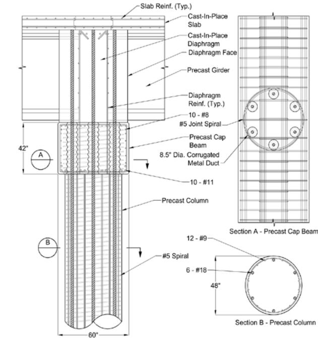
Fig. 5: Column to Cap Beam Connection
