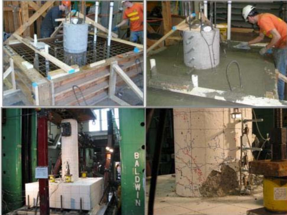
Fig. 8: UW Test setups for precast column-to-footing connection
