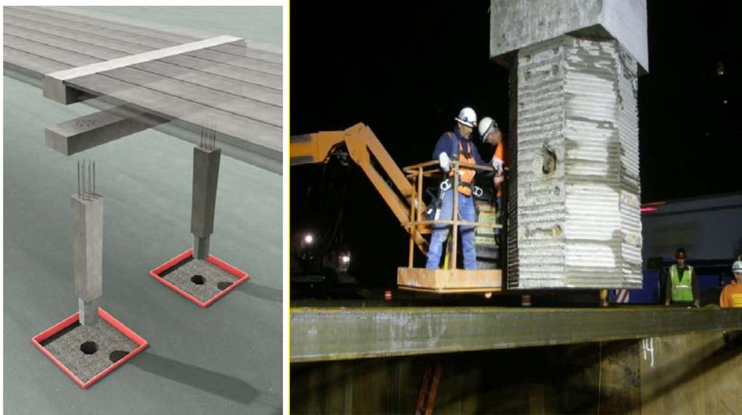
Fig. 3: Socket Connection Concept
