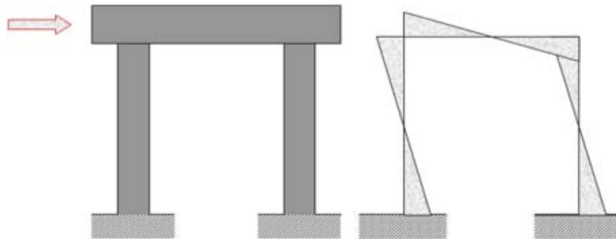
Fig. 1: Moment Diagram of a Bridge Pier with Fixed Connections
