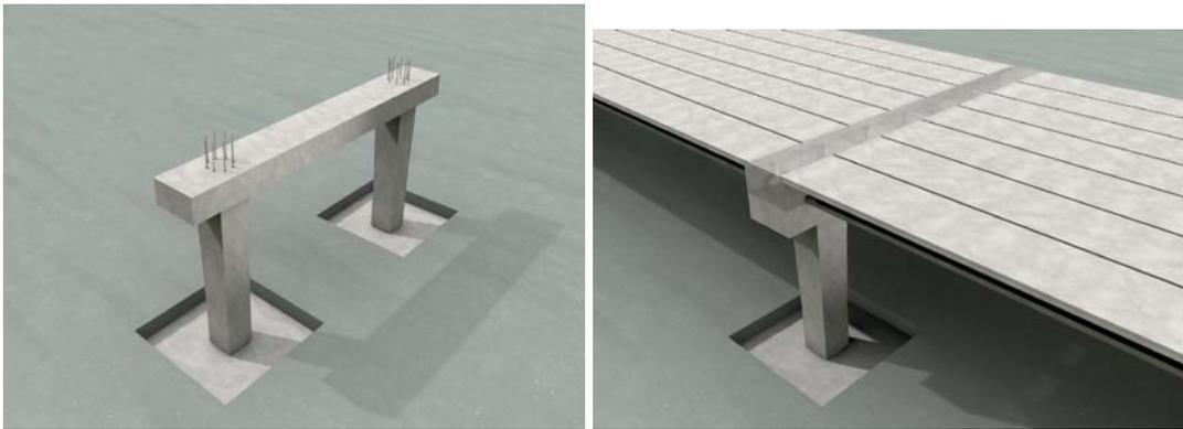
Fig 2: HfL System Configuration
