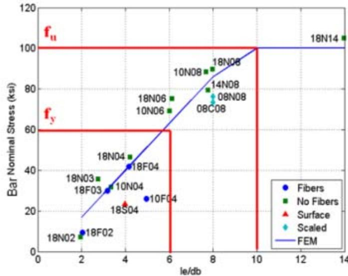
Fig. 6: UW Grouted Bar-Duct Pullout Test Results
