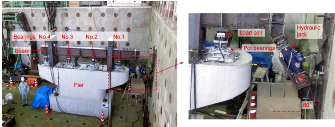
Fig. 6 Setup of loading test on large-scale bridge model
