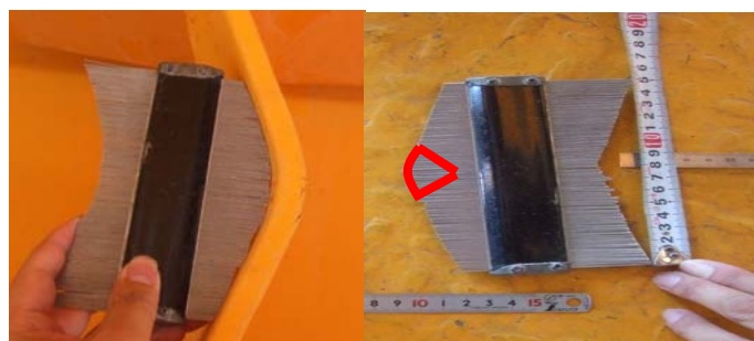
Figure 8 Surface curvature of bent plate
