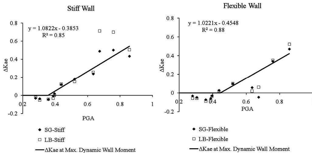
**Figure 9. Centrifuge Wall Modeling Results Illustrating when Dynamic Earth Pressure ( $\Delta K_{ae}$ ) Becomes Measurable (after Al Atik and Sitar, 2010).**
