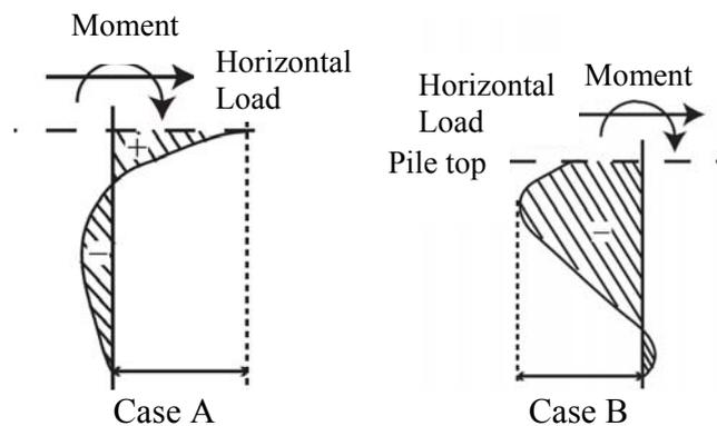
Figure 1 Bending moment distribution in a pile
