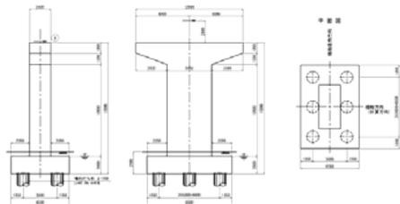
Case B ( $E_{PMT} = 8,400 \text{ kN/m}^2$ ,  $K_V = 687,000 \text{ kN/m}$ , Pile diameter,  $B = 1,350 \text{ mm}$ )
