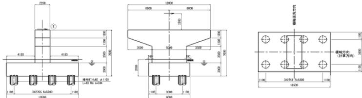
Case A ( $E_{PMT} = 1,400 \text{ kN/m}^2$ ,  $K_V = 580,000 \text{ kN/m}$ , Pile diameter,  $B = 1,100 \text{ mm}$ )
