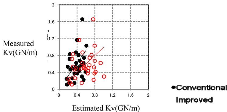
Figure 2 Estimated and Measured  $K_v$  relationships (Cast-in-place RC pile)
