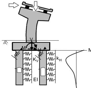
Figure 3 Design calculation model
