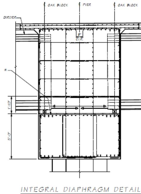
Figure 4: Lower Crossbeam Ties
