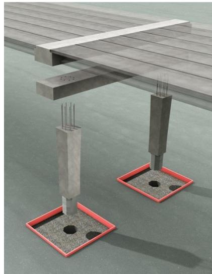
Figure 6. Precast concrete bent system configuration.
