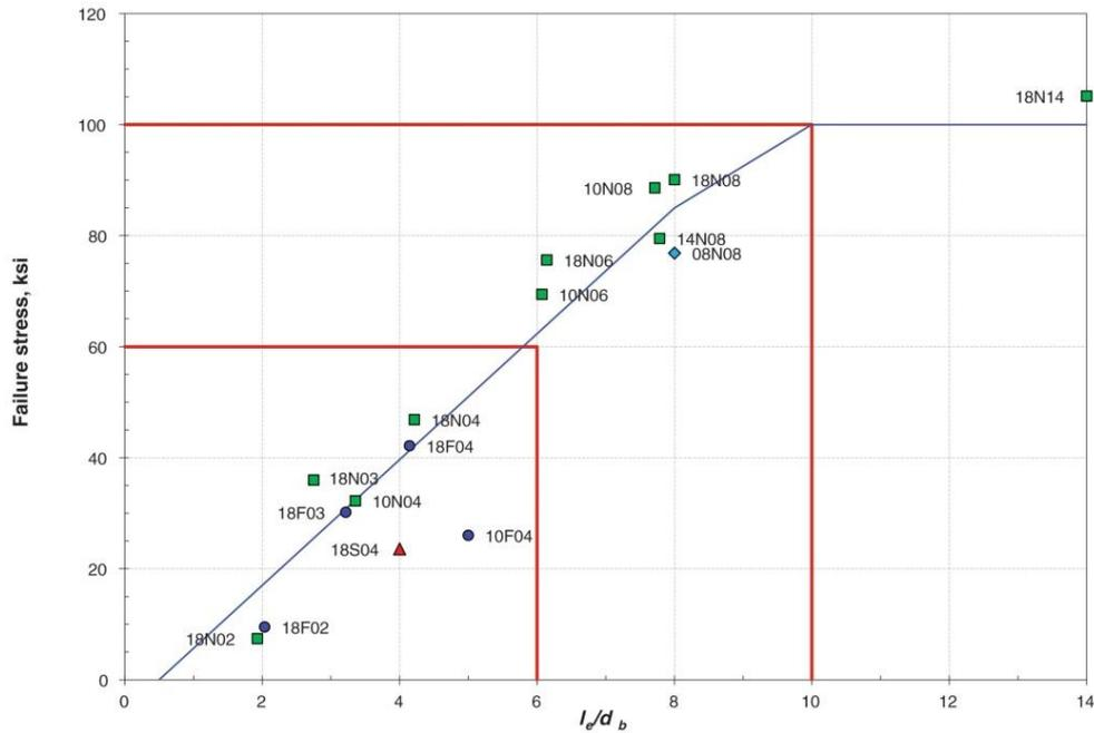
Figure 8. Grouted bar-duct pullout test results. Note:  $d_b$  = bar diameter;  $l_e$  = embedment length. 1 ksi = 6.895 MPa.
