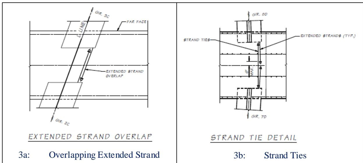
Figure 3: Overlapping Extended Strand and Strand Ties
