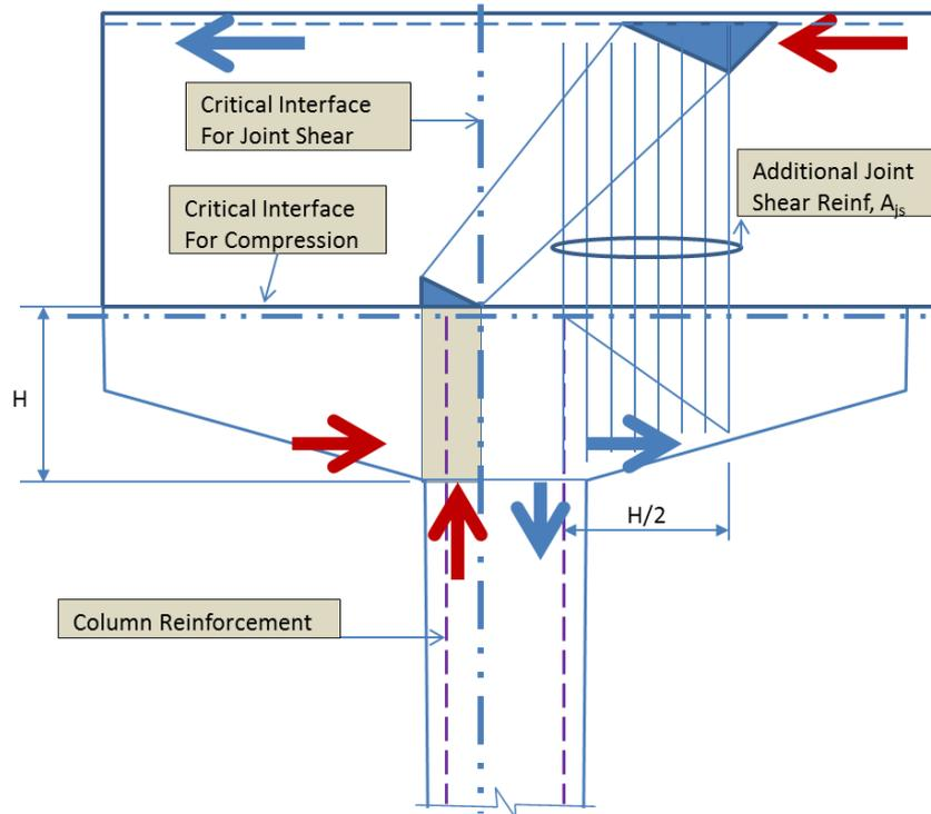
Figure 5: Strut and Tie Model of Intermediate Diaphragm
