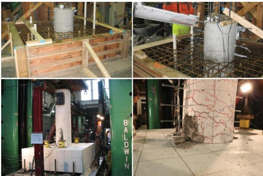
Figure 9. Construction and testing of precast concrete column-to-footing connection.
