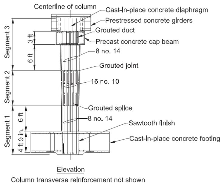
Figure 11. Demonstration bridge column details for elevation.
