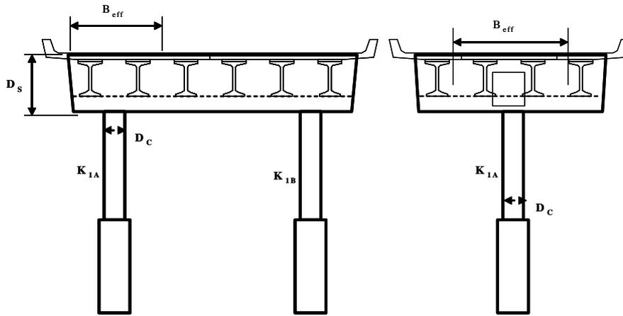
Figure 2: Effective Superstructure Width for Extended Strand Design
