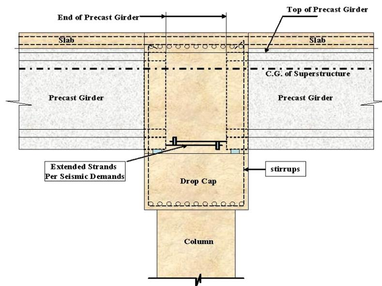
Figure 1: Pier with Girders Framed into the Pier Diaphragm
