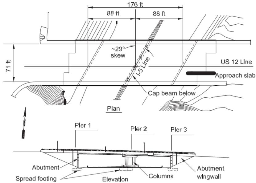
Figure 10. Bridge layout for demonstration project.
