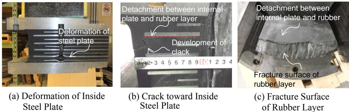
**Photo 4** Cut Section of As1-G1 Bearing
