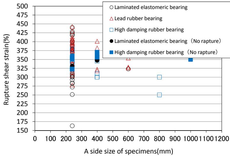
**Fig.1** Relation between rupture shear strain and a side size
