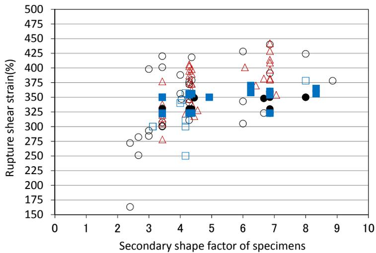
**Fig.2** Relation between rupture shear strain and secondary shape factor
