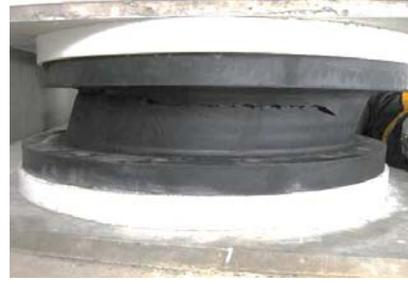
**Photo 2** Crack in Lead Rubber Bearing
