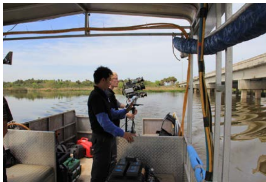
Fig.10: Digital image scanning from a pontoon boat
