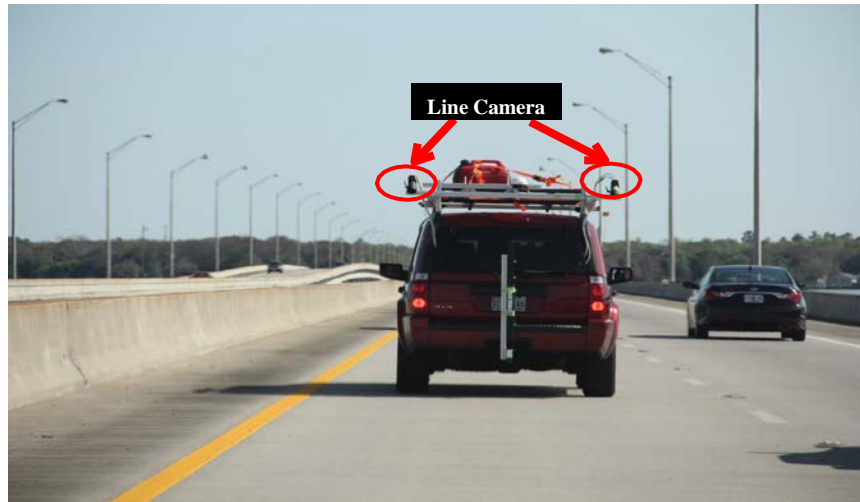
Fig.4: Digital image scanning for deck top from a moving vehicle
