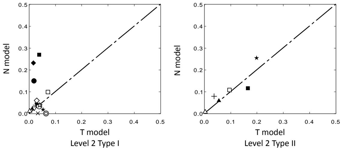
Figure 9 Comparison of the residual displacements of T and N models.
