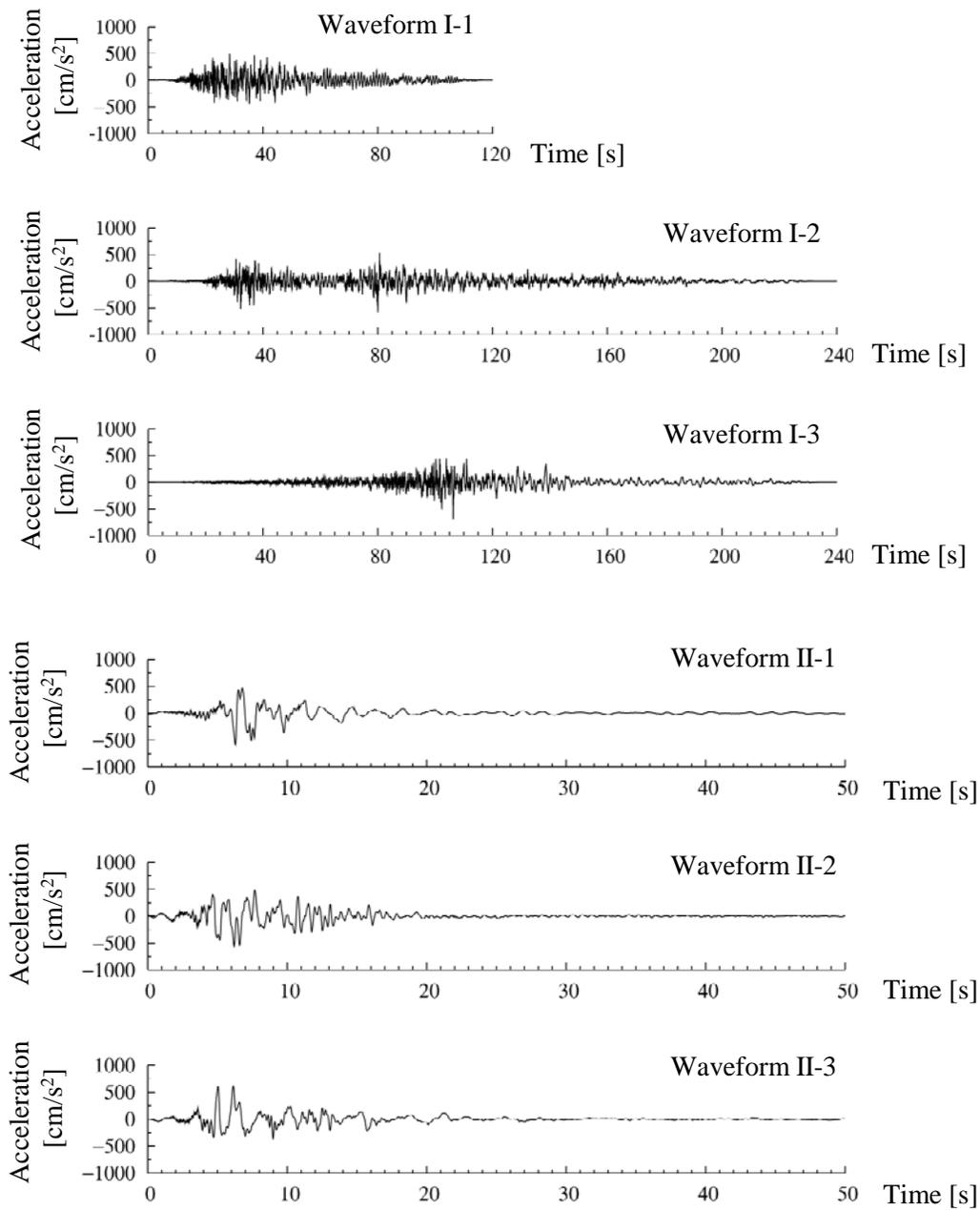
Figure 1 Waveforms used for the nonlinear dynamic analyses. Waveforms I-1, I-2 and I-3 are earthquake motions at Type III ground from large-scale plate boundary earthquakes, while waveforms II-1, II-2 and II-3 are those from inland earthquakes.
