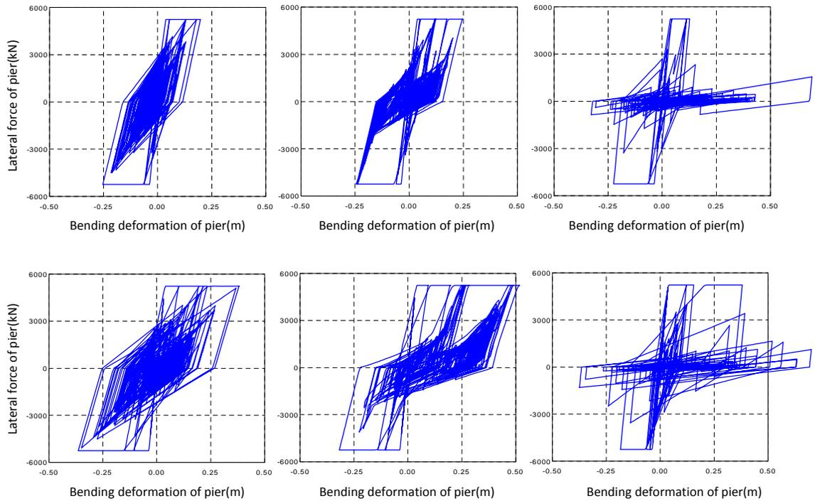
Figure 7 Hysteresis response of the RC pier subjected to the waveform I-2 (top: x1.0, bottom: x2.0).
