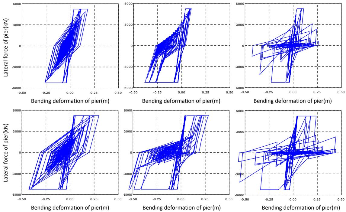
Figure 6 Hysteresis response of the RC pier subjected to the waveform I-1 (top: x1.5, bottom: x2.0)
