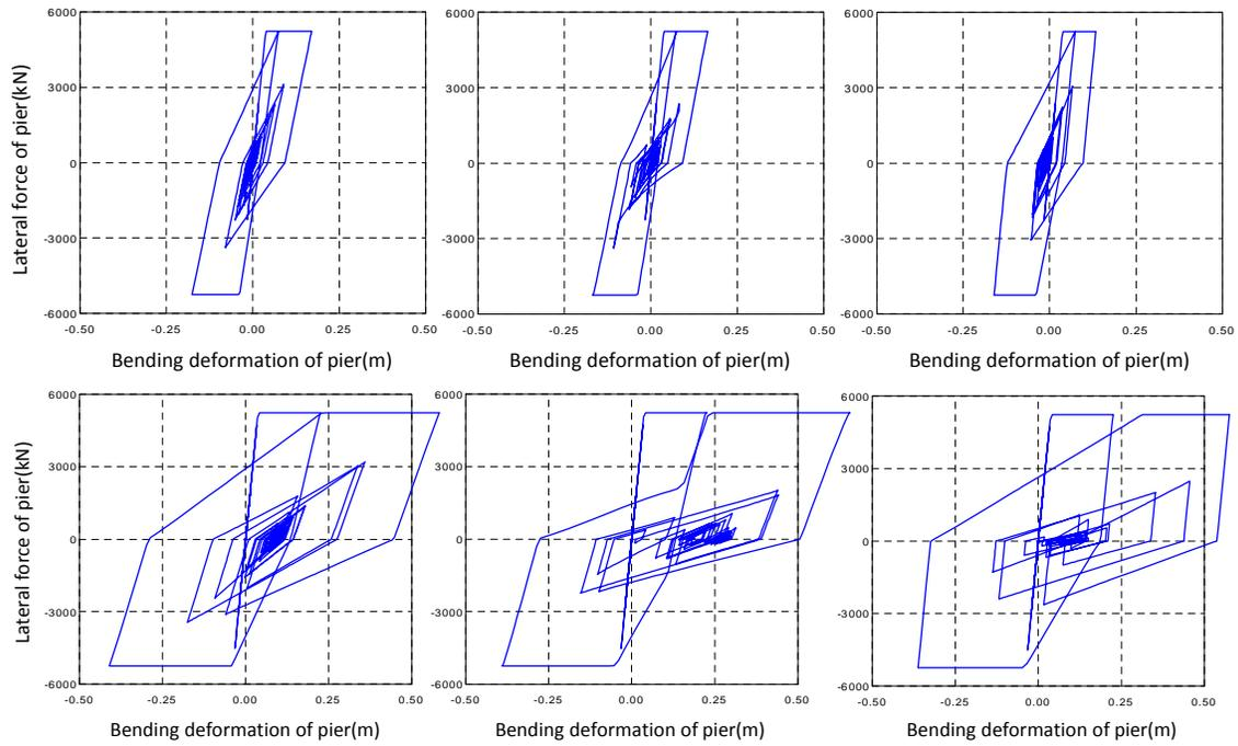
Figure 5 Hysteresis response of the RC pier subjected to the waveform II-1 (top: x1.0, bottom: x2.0).
