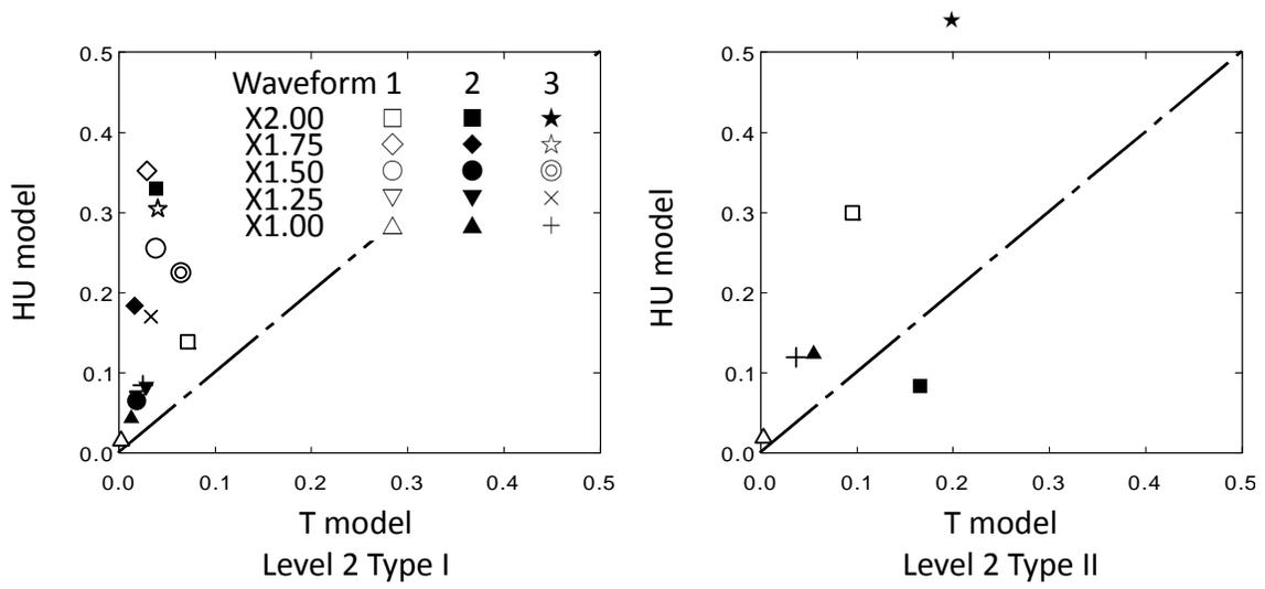
Figure 8 Comparison of the residual displacements of T and HU models.
