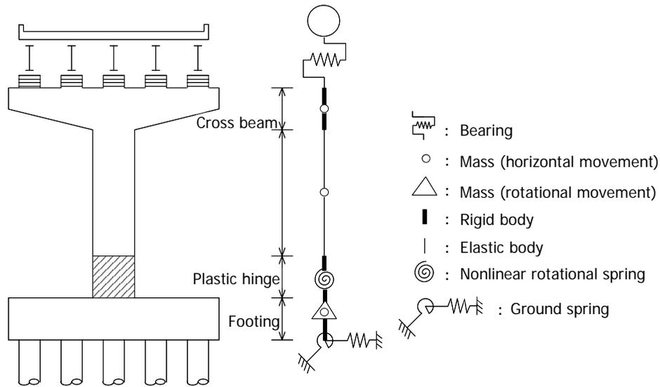
Figure 2 Analytical model of a highway bridge.
