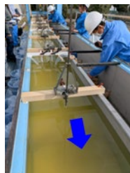
Water-level measurement and water sampling at multiple locations along the flume
