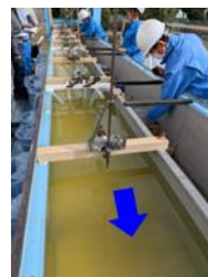
Water level and water sampling at multiple locations along the flume
