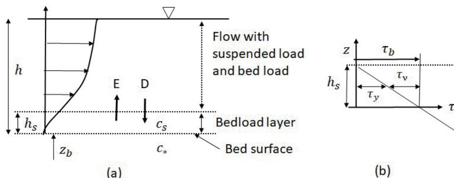
Figure 3 Schematic diagram showing (a) definition of flow field and (b) constitutive relation in bed load layer
