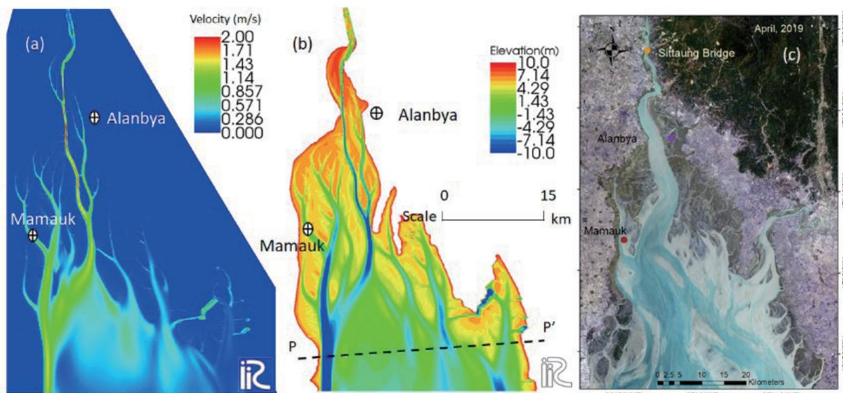
Figure 5 (a) Computed spatial distribution of velocity during ebb tide, (b) computed bed evolution and (c) comparison of results with Landsat 8 satellite image on April, 2019
