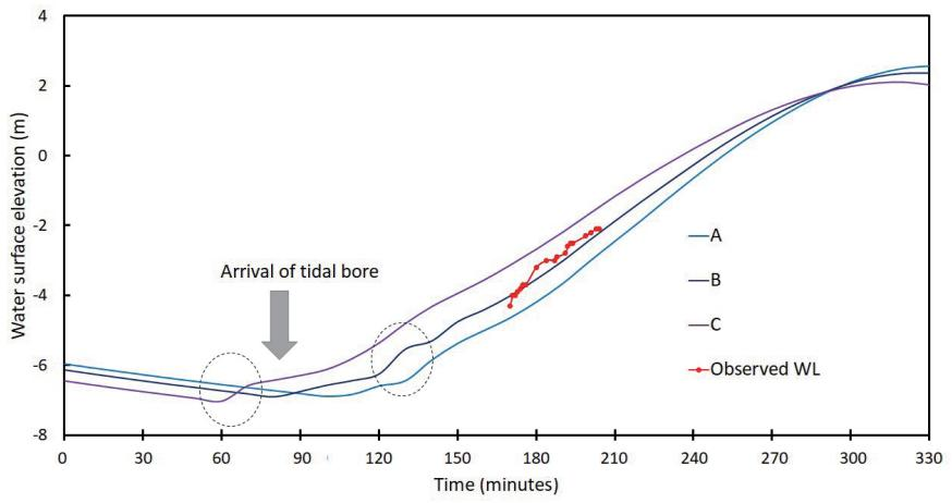
Figure 4 Temporal change of computed water surface elevations at sites near Mamauk and comparison with observed data
