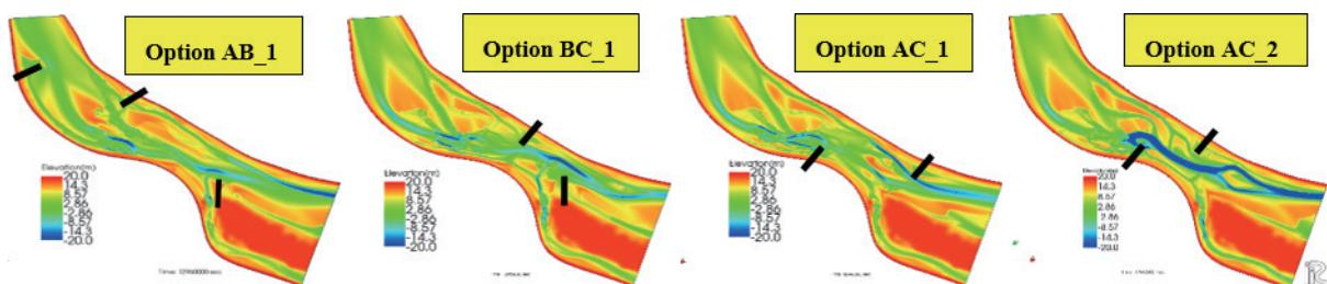
Figure: Computed results for the different series of countermeasures at around the Gorai river off-take area. The color contour shows the elevation.
