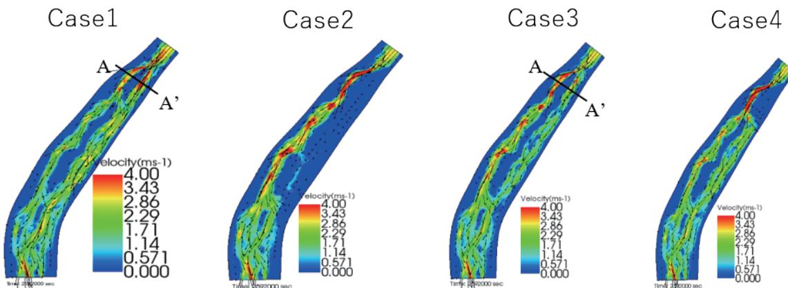
Figure: Computed results for the different series of countermeasures. The color contour shows the velocity distributions.
