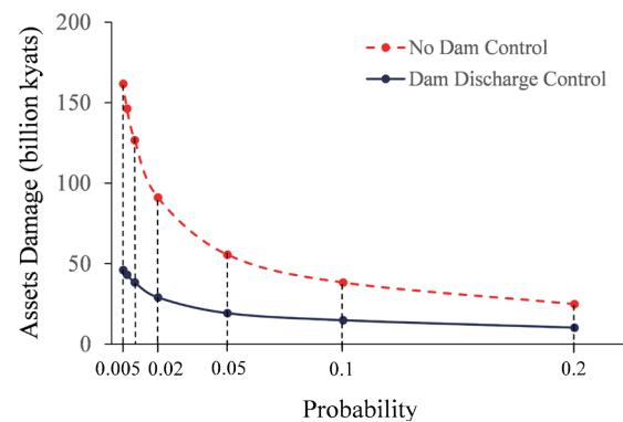
Figure 3 Damage-probability curves for assets damage with (discharge control rate: 500 m<sup>3</sup>/s) and without flood-control dam operation at the ZTD [2].
