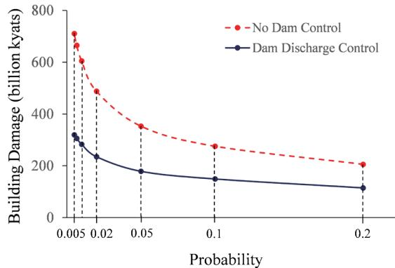
Figure 2 Damage-probability curves for building damage with (discharge control rate: 500 m<sup>3</sup>/s) and without flood-control dam operation at the ZTD [2].
