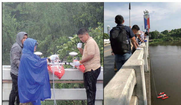
Figure 2. Field training on ADCP deployment over bridge in June 2024
