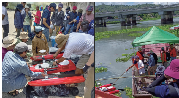
Figure 1. Field training on ADCP deployment by boat in May 2024.
