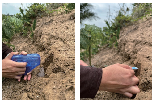
Photo 4 Field investigation on riverbank erodibility
