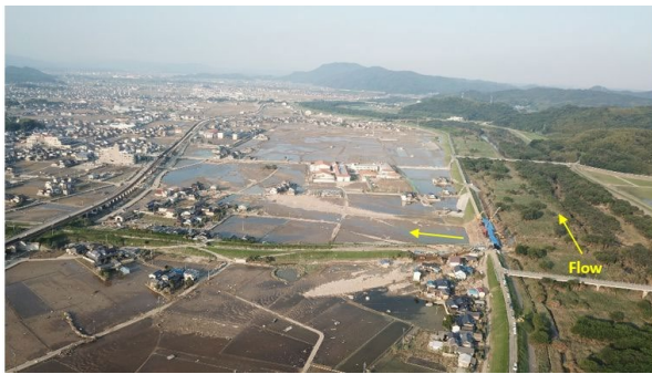
Photo 4-1 Levee breach along the Oda River (a drone photo taken over Mabi Town, Kurashiki City)
