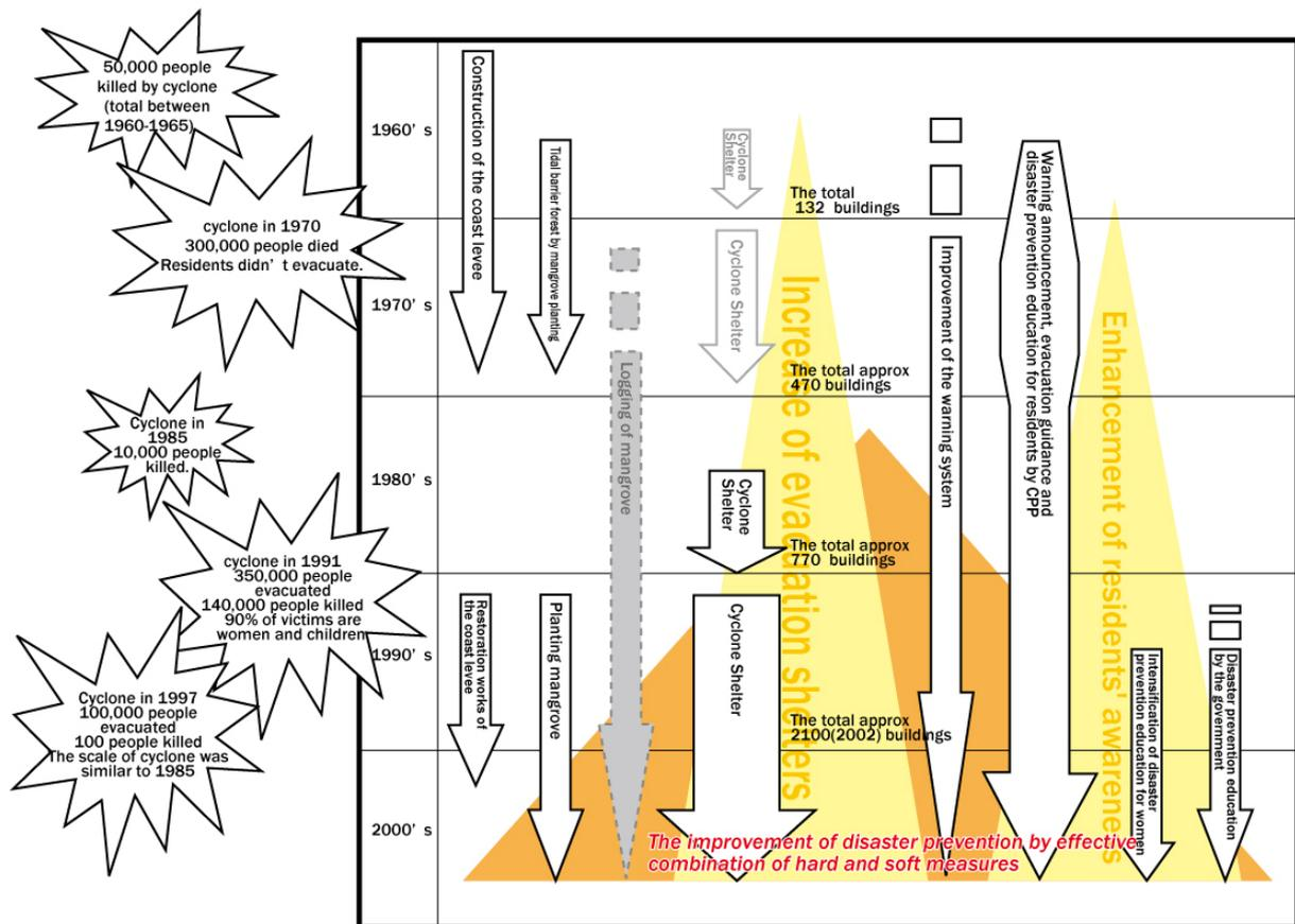
**Fig 28: History of cyclonic damage and prevention measures**
