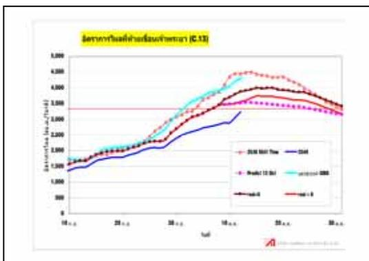
The volume of water passing through the lower Chao Phraya dam is forecasted to be 3,800 cubic meters. With regard to the tide, I have used the tidal pattern of the last two months to forecast the tidal behavior for the next month.
