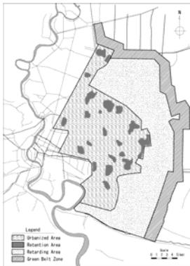
**Fig. 29 Green Belt, Retarding Area and Retention Area as Non-Structural Measures**
