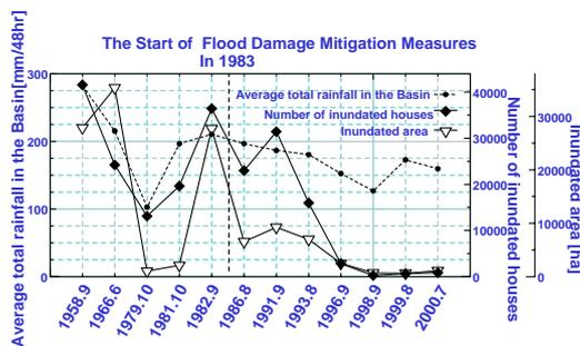
Fig. 16 Changes of Inundated Areas and Houses at Time of Recorded Flooding in the Naka River/Ayase River Basin
