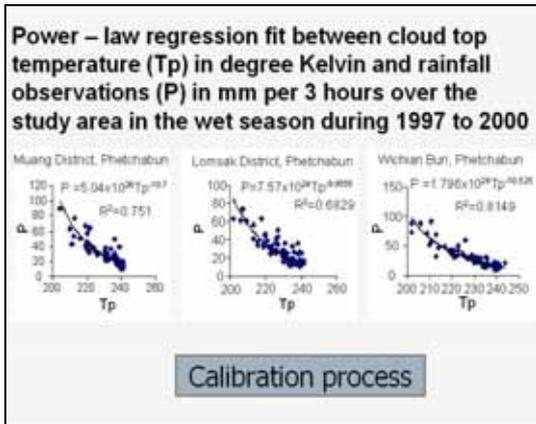
The calibration process by using the power-law regression fits between the cloud top temperature, (TP, in degree Kelvin) and rainfall observation, (P in millimeter per three hours) over the study area during the wet season from 1997 to 2000.
