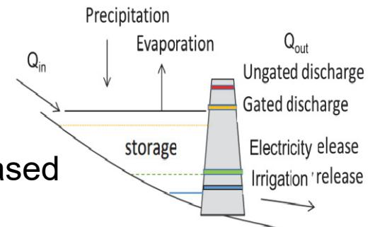
The BTOP Dam module determines irrigated area based on reservoir water volume and calculates daily discharge using
